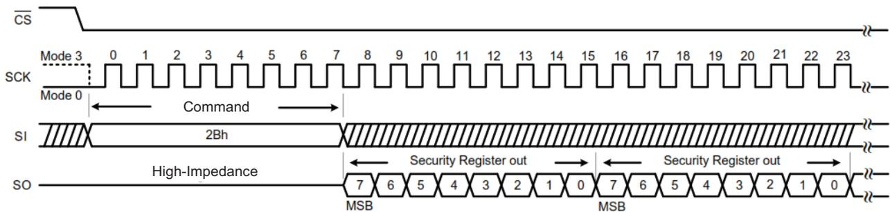
**Figure 64. Read Security Register Command (QPI Mode)**
