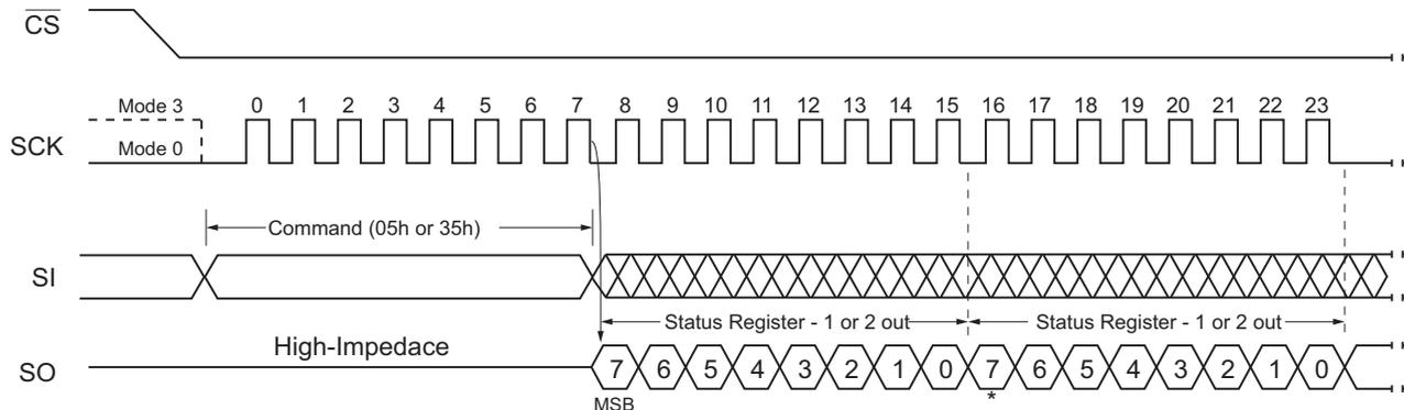
Figure 10. Read Status Register Command (QPI Mode)
