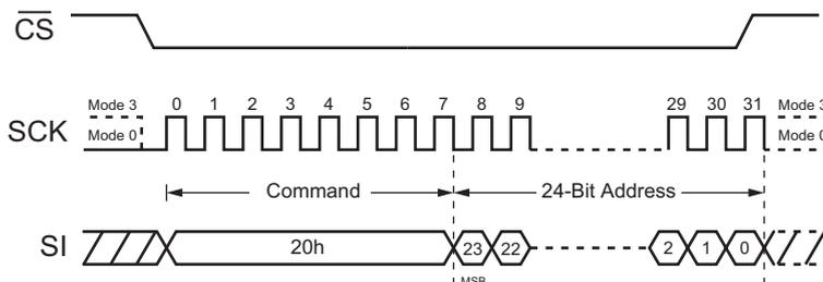
Figure 31. Block Erase Command (QPI Mode)
