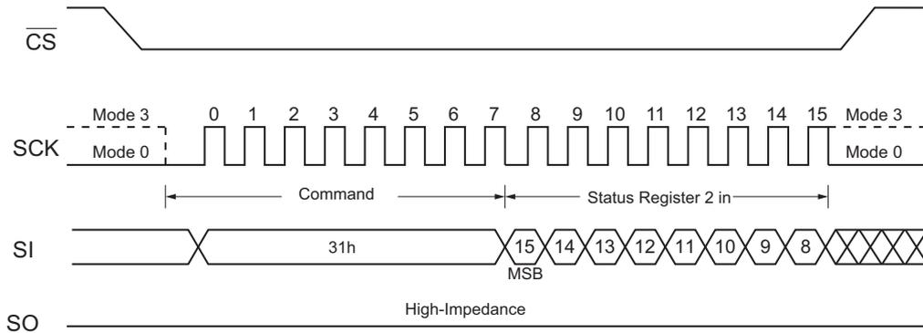
Figure 14. Write Status Register-2 Command (QPI Mode)
