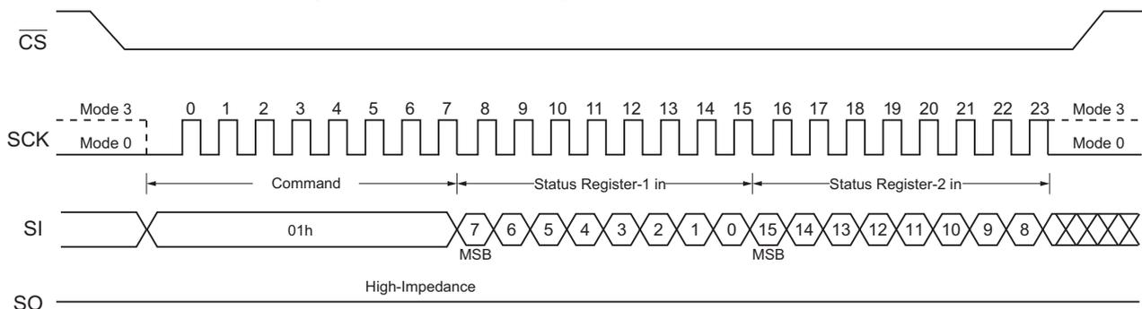
Figure 12. Write Status Register Command (QPI Mode)
