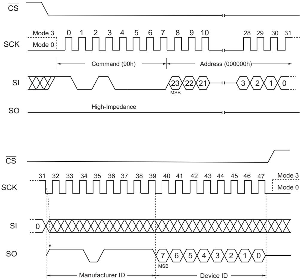
Figure 47. Read Manufacturer/ Device ID Command (QPI Mode)
