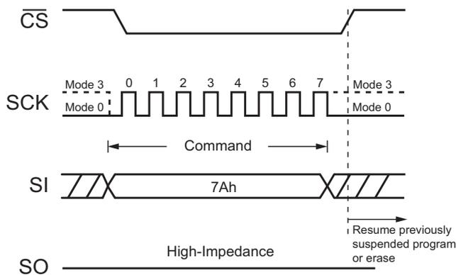
Figure 40. Erase / Program Resume Command (QPI Mode)
