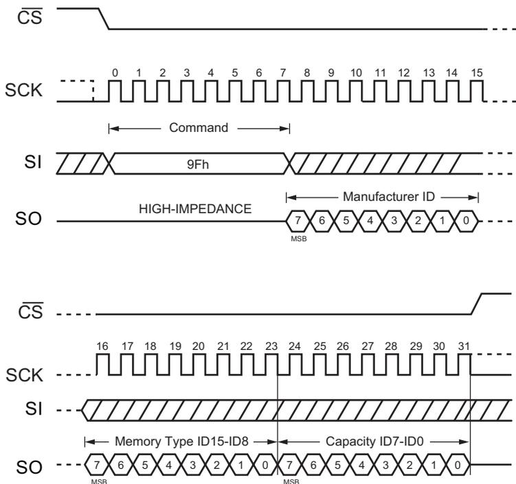
Figure 51. Read JEDEC ID Command (QPI Mode)
