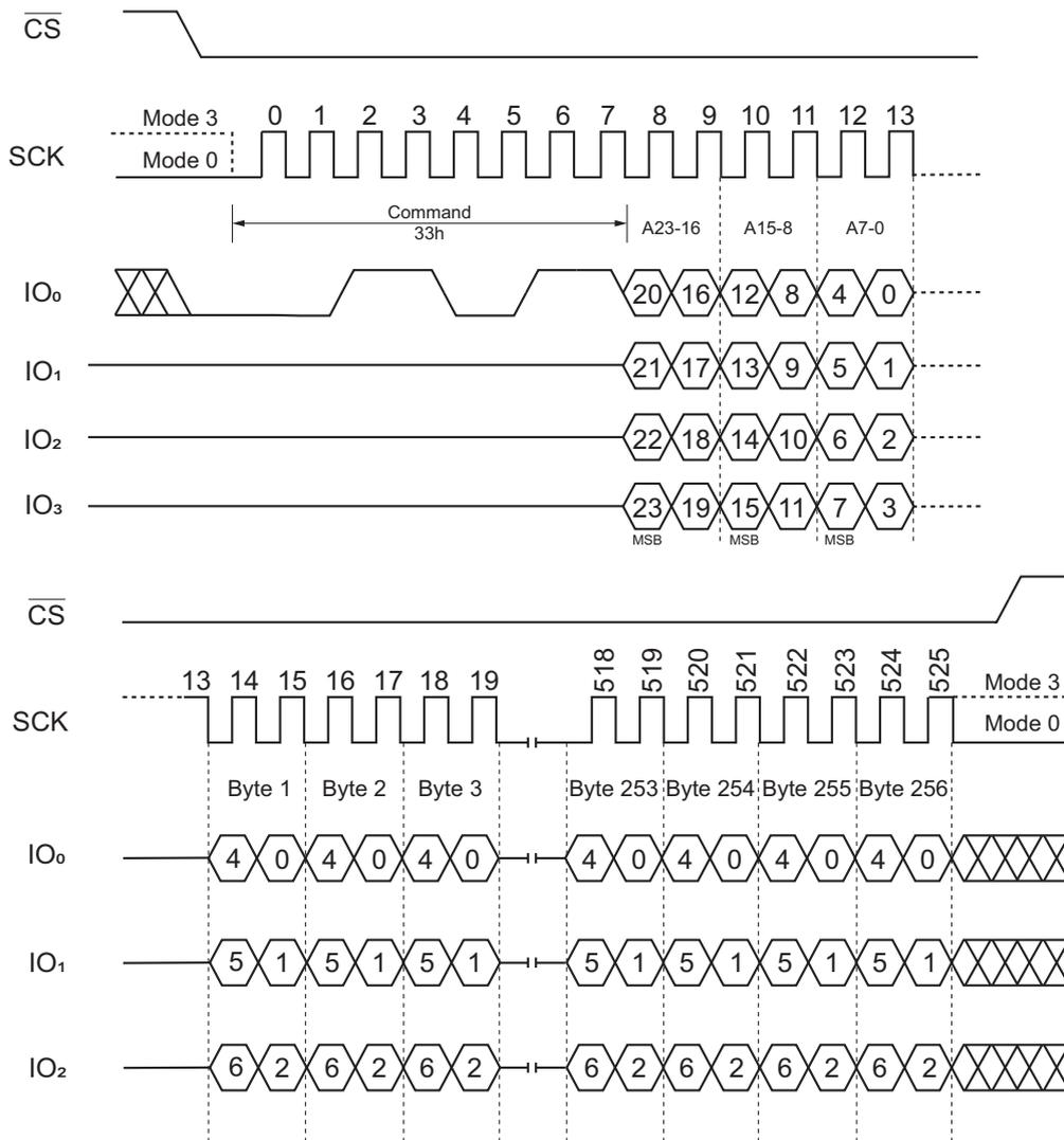
Figure 29. Quad Page Program Command (QPI mode)
