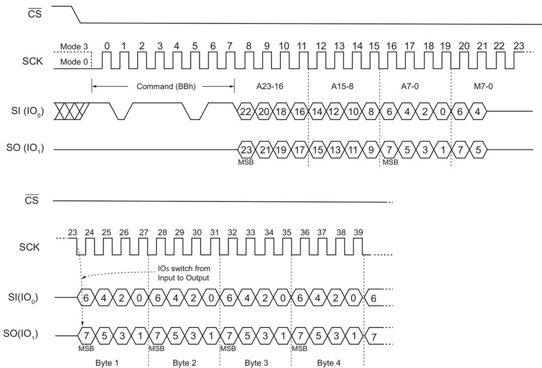
Figure 22. Fast Read Dual I/O Command (previous M7-0= Axh)
