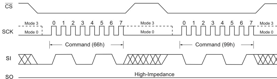
Figure 59. Enable Reset and Reset Command (QPI Mode)
