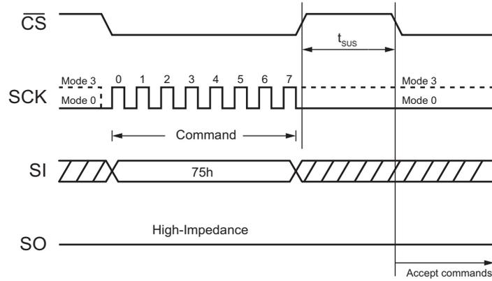
**Figure 38. Erase Suspend Command (QPI Mode)**
