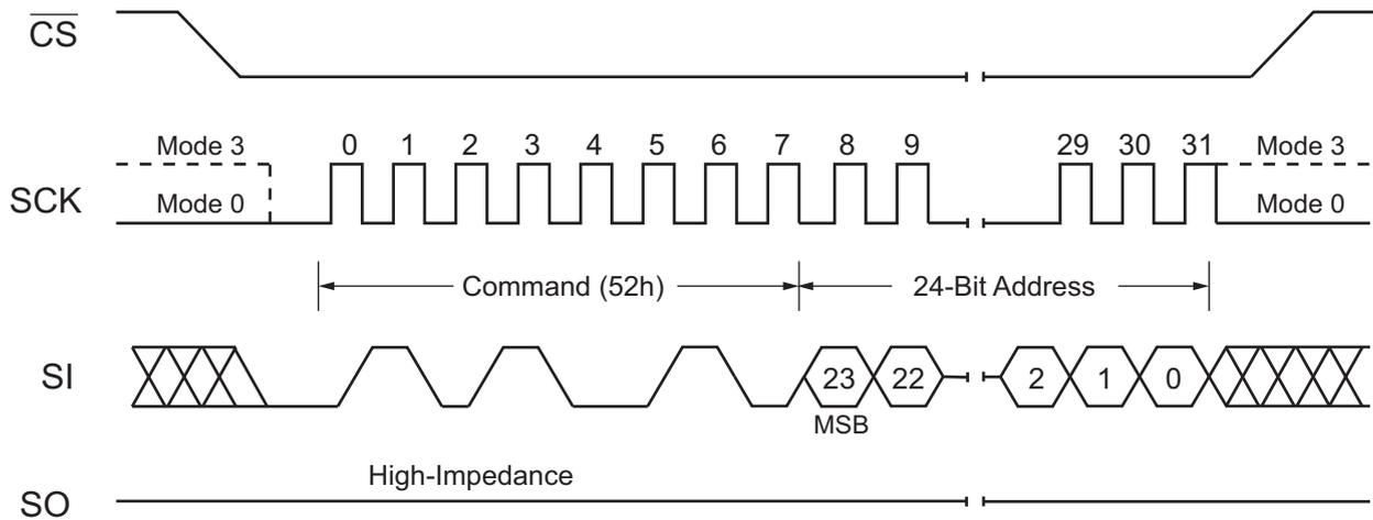
Figure 33. 32 kB Block Erase Command (QPI Mode)
