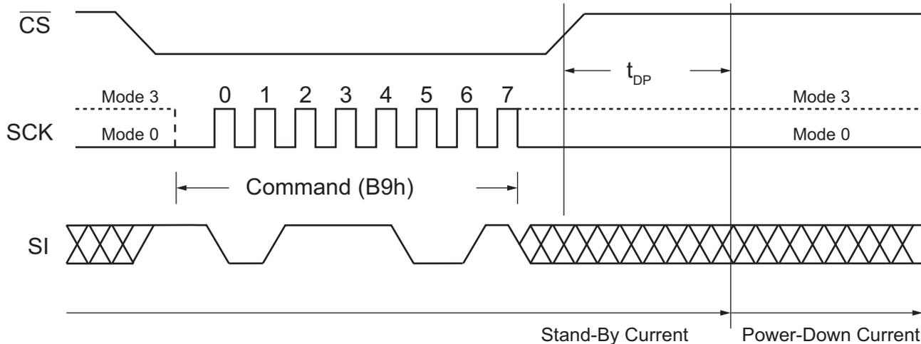
Figure 42. Deep Power-Down Command (QPI Mode)
