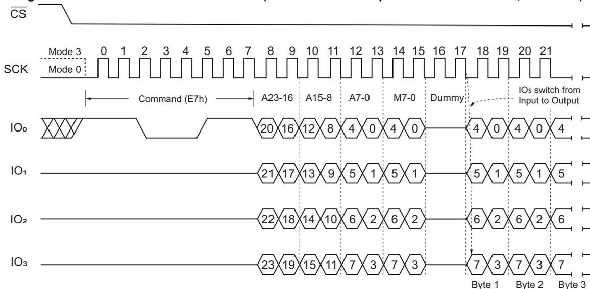
Figure 55. Word Read Quad I/O Command (Previous command set M7-0 = Ah, SPI Mode)
