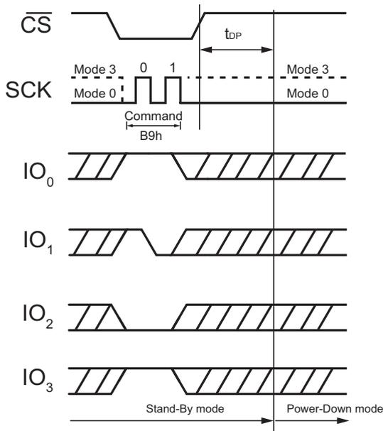
Figure 45. Release Power-Down / Device ID Command (SPI Mode)
