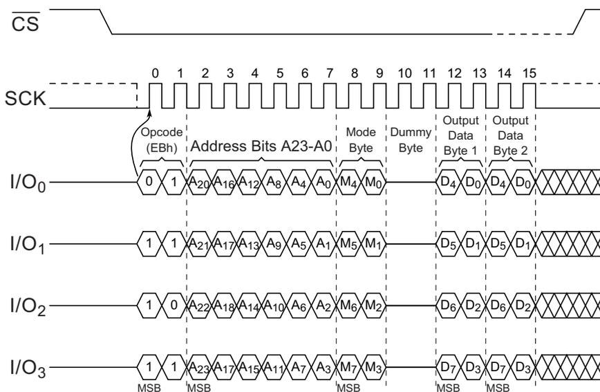
Figure 25. Fast Read Quad I/O Command (Initial command or previous M7-0 ≠ Axh, QPI mode, 80 MHz)
