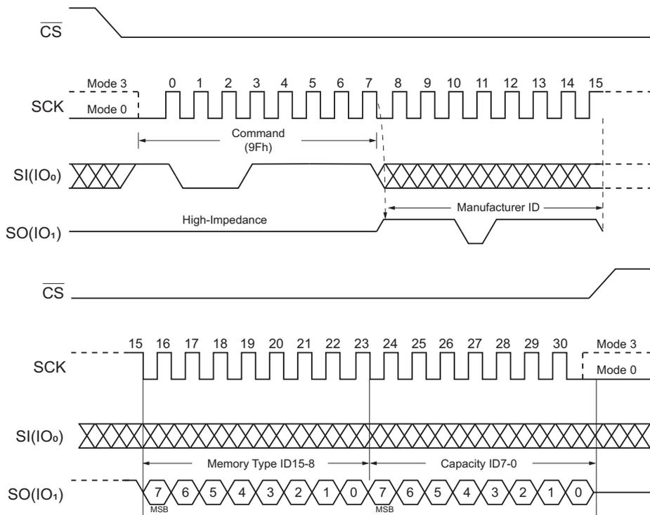
Figure 51. Read JEDEC ID Command (SPI Mode)
