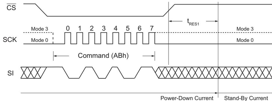
Figure 44. Release Power-Down Command (SPI Mode)
