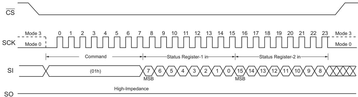
Figure 11. Write Status Register Command (SPI Mode)
