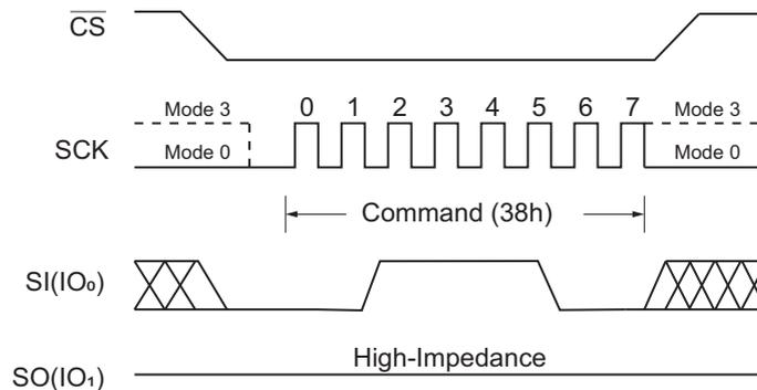
Figure 53. Enable QPI Command (SPI Mode only)
