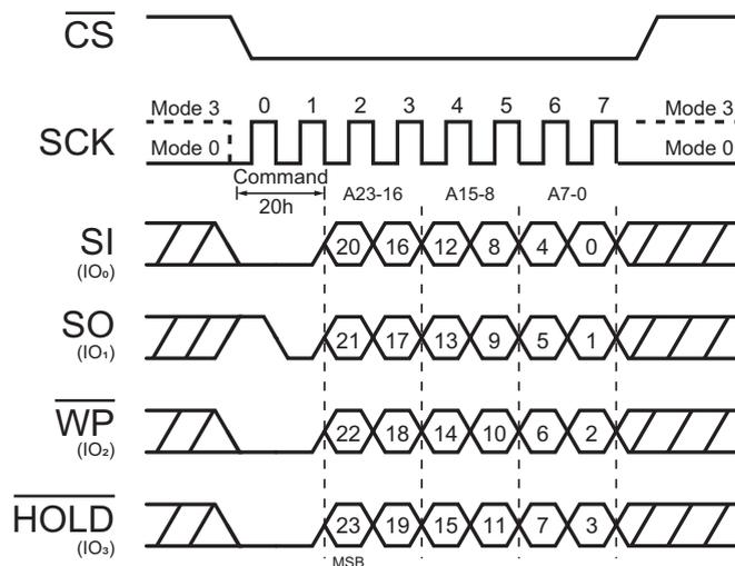
Figure 32. Block Erase Command (QPI Mode)
