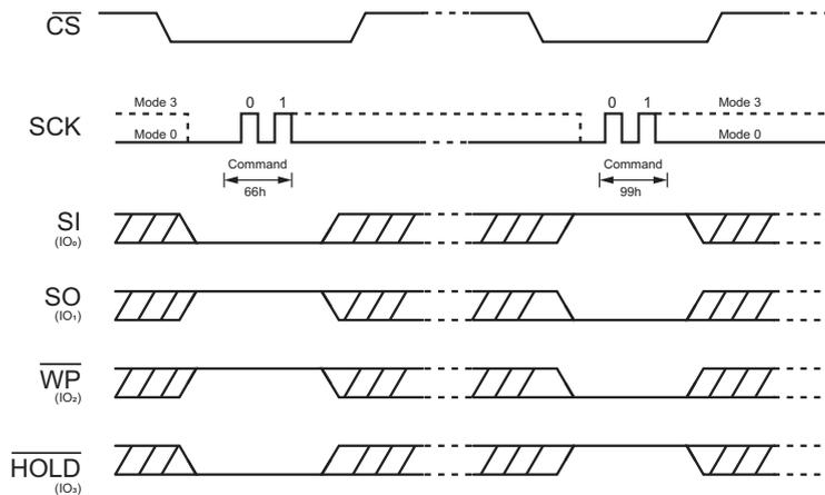
Figure 62. Enable Reset and Reset Command (QPI Mode)
