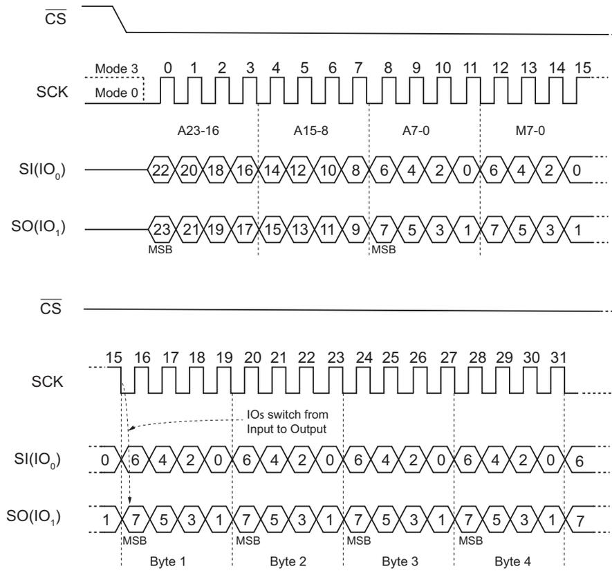
Figure 22. Fast Read Dual I/O Command (previous M7-0 = A<sub>xh</sub>)
