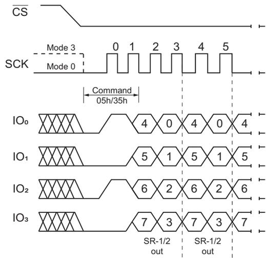
Figure 10. Read Status Register Command (QPI Mode)
