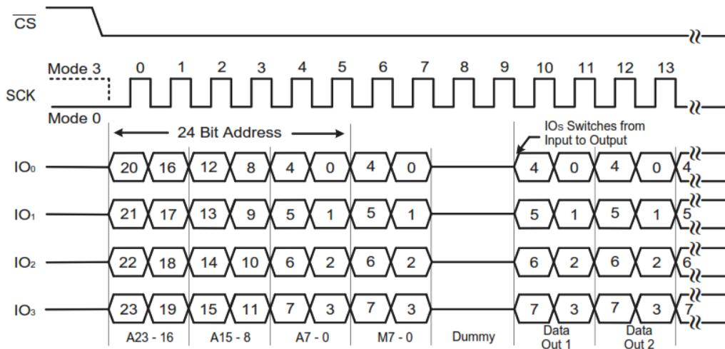
Figure 57. Set Burst with Wrap Command Sequence
