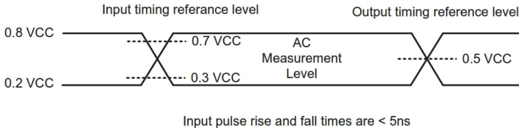
Figure 70. AC Measurement I/O Waveform
