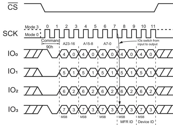
Figure 48. Read Manufacturer/ Device ID Command (QPI Mode)
