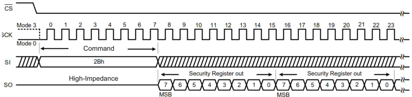
Figure 66. Read Security Register Command (SPI Mode)
