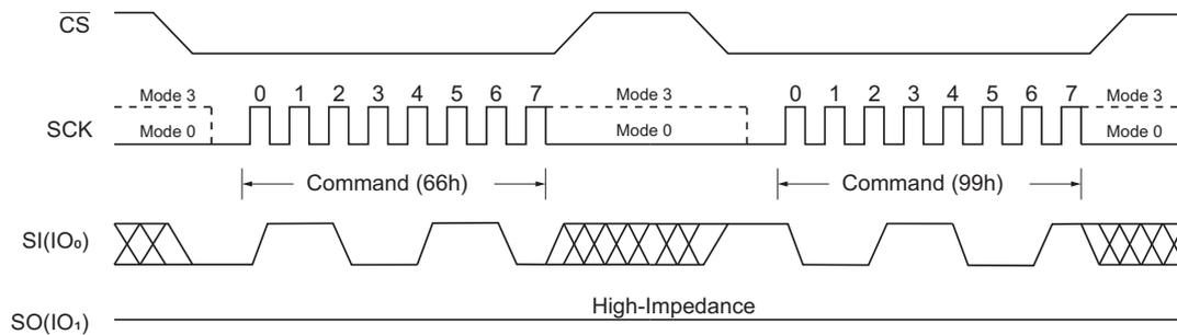
Figure 61. Enable Reset and Reset Command (SPI Mode)
