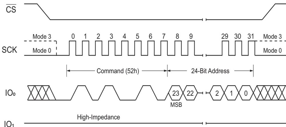
Figure 33. 32 kbytes Block Erase Command (SPI Mode)
