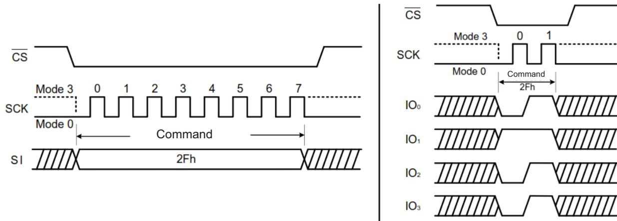
Figure 68. Write Security Register Command for SPI Mode (left) and QPI Mode (right)
