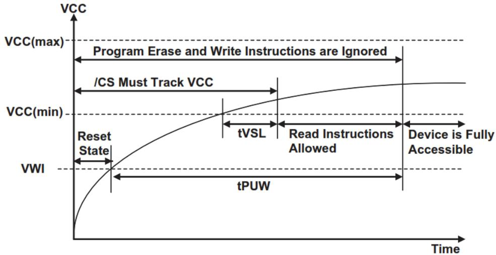
Figure 69. Power-Up Timing and Voltage Levels
