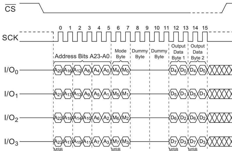
Figure 24. Fast Read Quad I/O Command (previous M7-0 = Axh, SPI mode)
