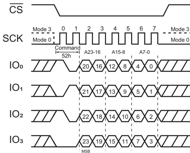
Figure 34. 32 kbytes Block Erase Command (QPI Mode)
