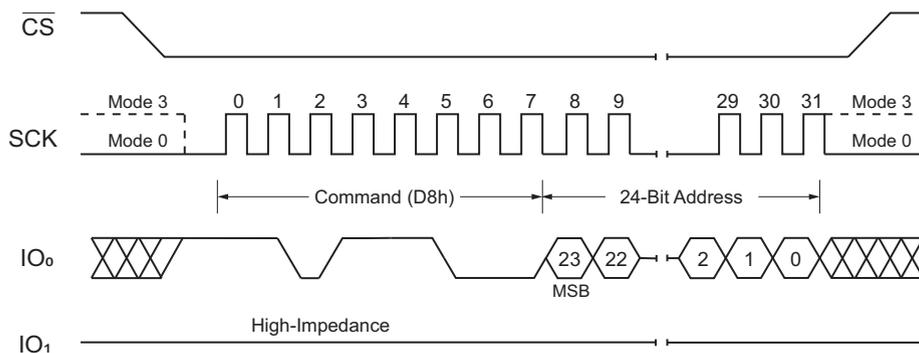
Figure 35. 64 kbytes Block Erase Command (SPI Mode)
