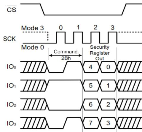
Figure 67. Read Security Register Command (QPI Mode)
