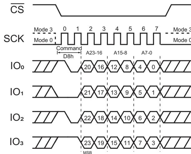
Figure 36. 64 kbytes Block Erase Command (QPI Mode)
