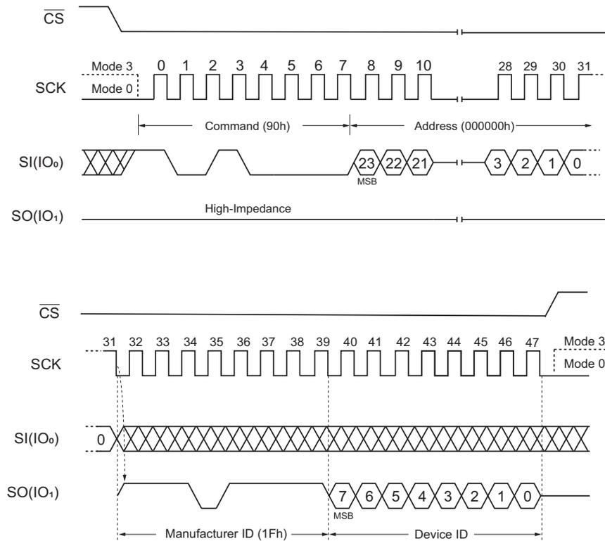
Figure 47. Read Manufacturer/ Device ID Command (SPI Mode)
