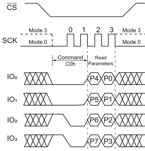
Figure 60. Set Read Parameters command (QPI Mode)
