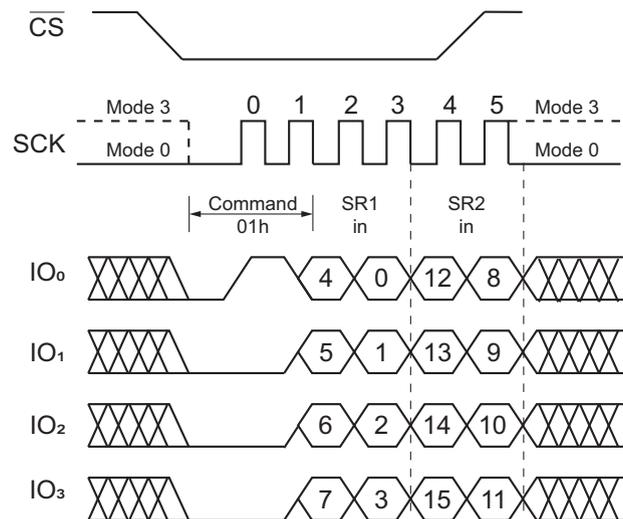
Figure 12. Write Status Register Command (QPI Mode)
