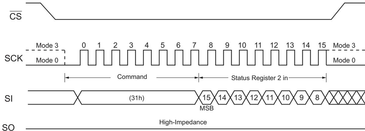
Figure 13. Write Status Register-2 Command (SPI Mode)
