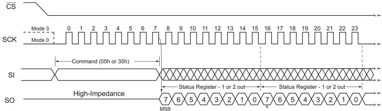
Figure 9. Read Status Register Command (SPI Mode)
