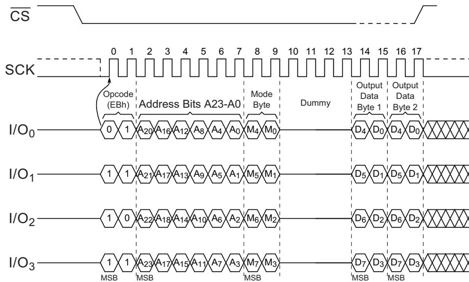
Figure 26. Fast Read Quad I/O Command (Initial command or previous M7-0 ≠ A<sub>xh</sub>, QPI mode, 133 MHz)
