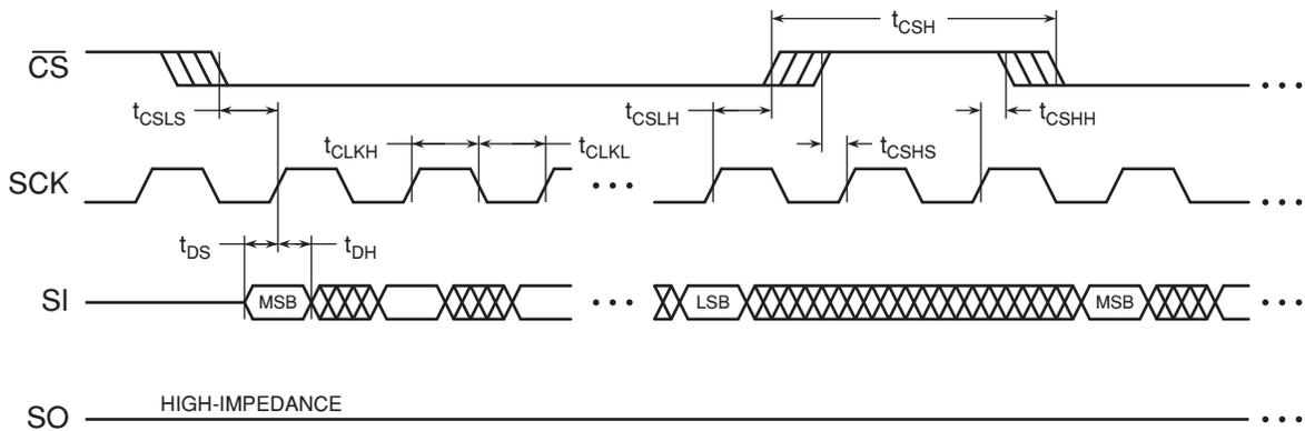
Figure 14-2. Serial Output Timing
