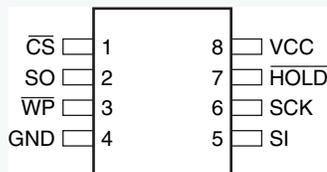
**Figure 2-3. 8-UDFN (Top View)**
