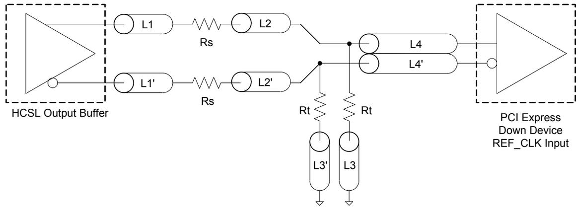
Figure 2: Differential Routing to PCI Express Controller
