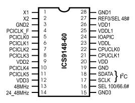
28 pin SOIC and SSOP
