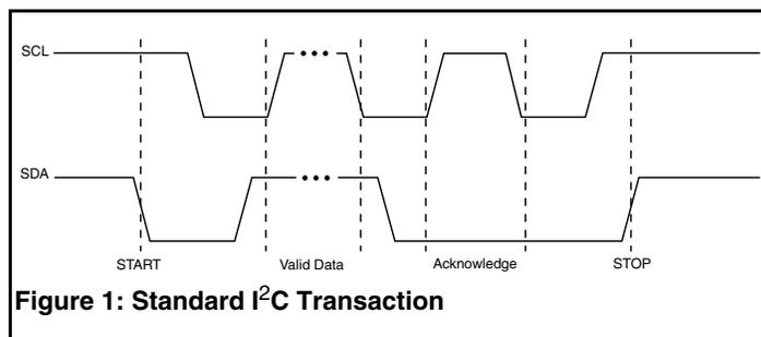
**Figure 1: Standard I<sup>2</sup>C Transaction**
