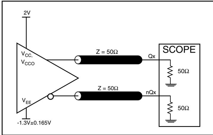
3.3 Core/3.3V LVPECL Output Load AC Test Circuit
