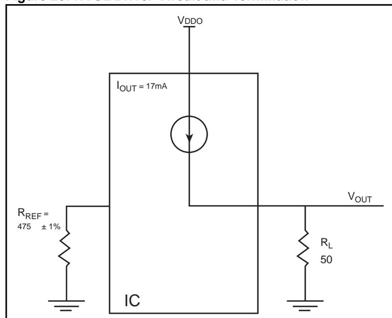
HCSL is a current steering output which sources a maximum of 17mA of current per output. To calculate worst case on-chip power dissipation, use the following equations which assume a 50Ω load to ground.
