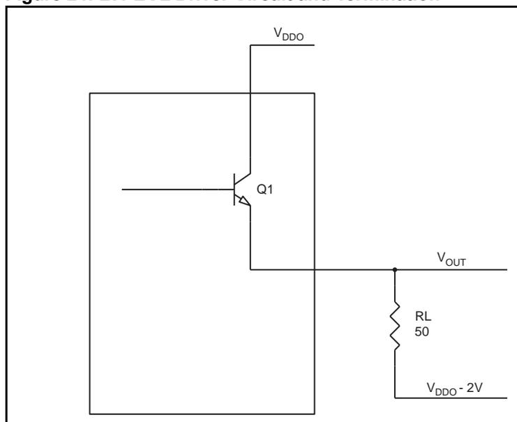
To calculate power dissipation per output pair due to loading, use the following equations which assume a 50Ω load, and a termination voltage of  $V_{DDO} - 2V$ .
