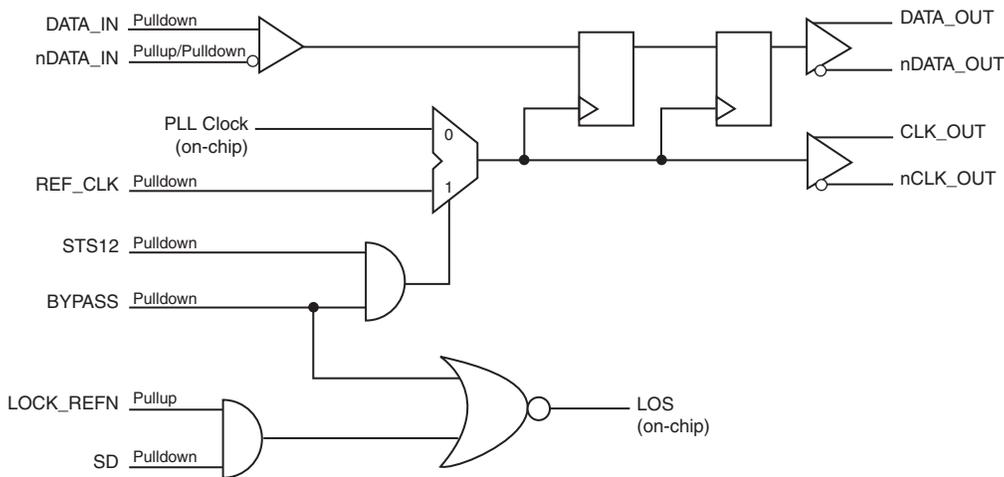
**Figure 1. Signal Detect/PLL Bypass Operation Control Diagram**
