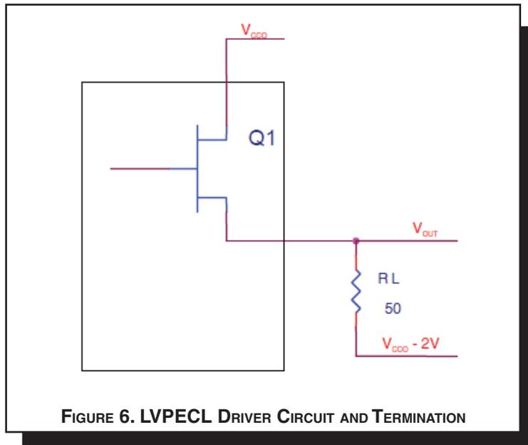
To calculate worst case power dissipation into the load, use the following equations which assume a 50Ω load, and a termination voltage of  $V_{CCO} - 2V$ .
