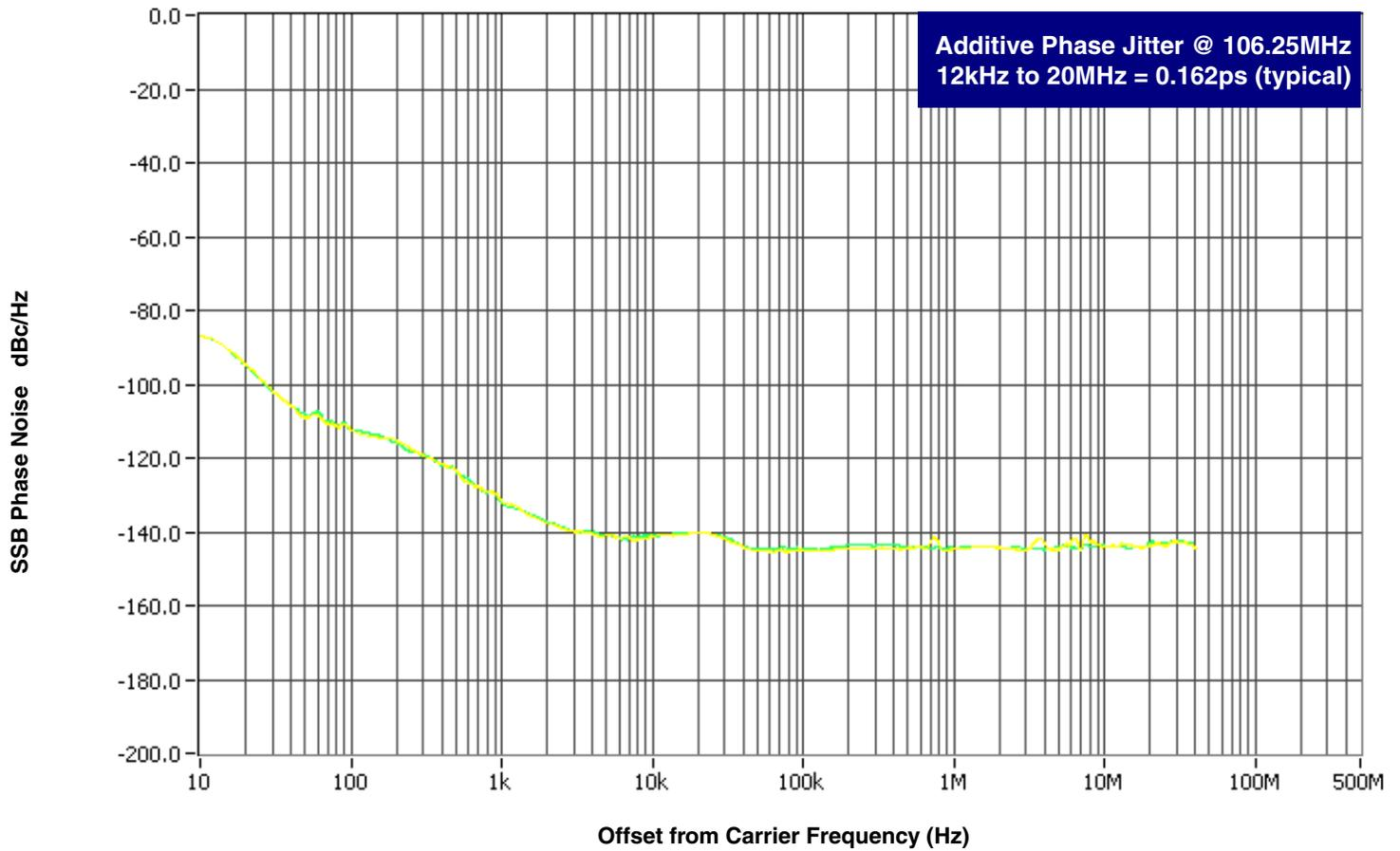
As with most timing specifications, phase noise measurements has issues relating to the limitations of the equipment. Often the noise floor of the equipment is higher than the noise floor of the device. This
