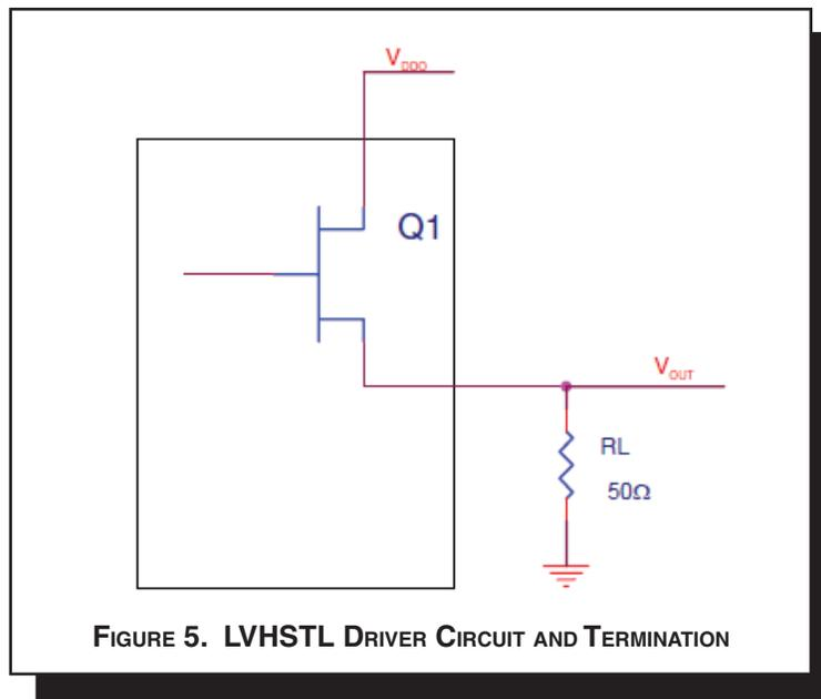
**FIGURE 5. LVHSTL DRIVER CIRCUIT AND TERMINATION**
