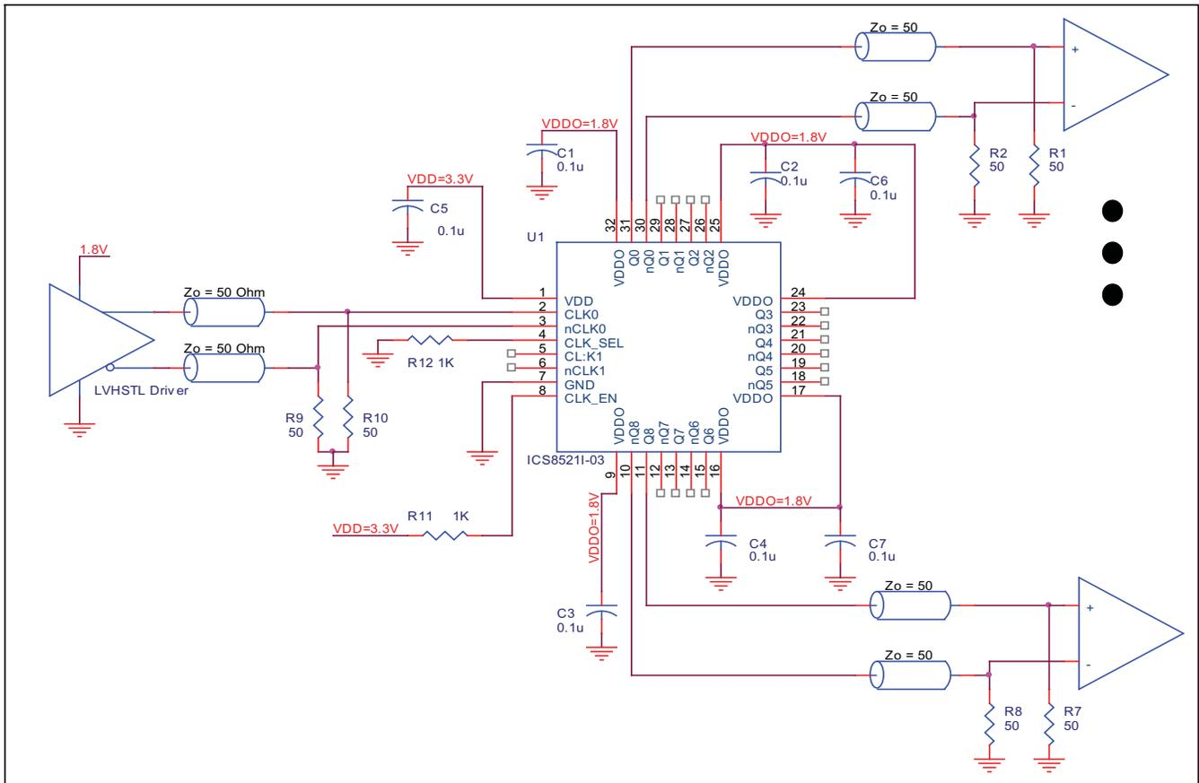
FIGURE 3B. RECOMMENDED LAYOUT OF BYPASS CAPACITOR PLACEMENT
