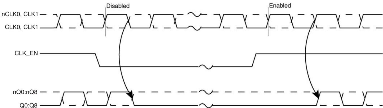
**FIGURE 1. CLK\_EN TIMING DIAGRAM****TABLE 3B. CLOCK INPUT FUNCTION TABLE**
