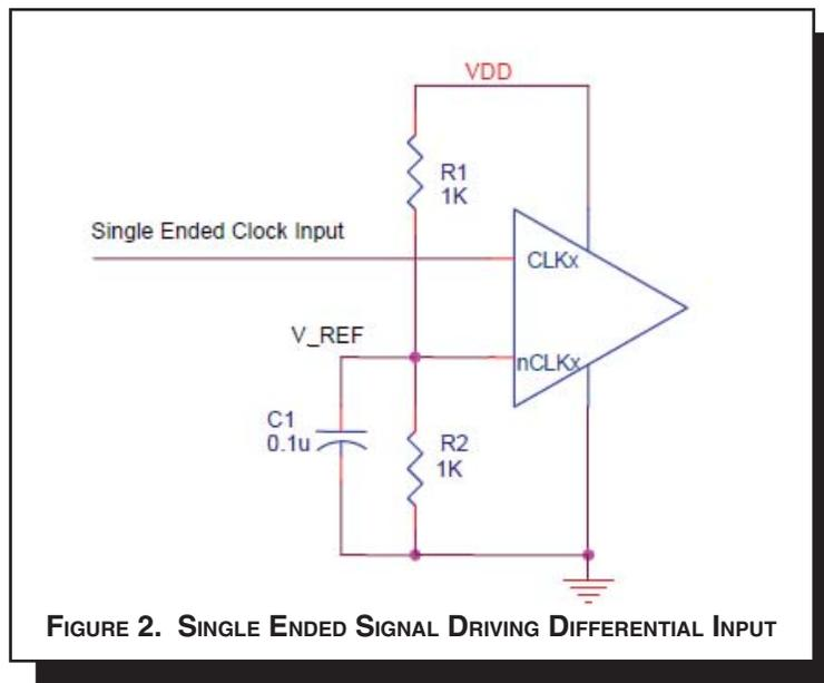
FIGURE 2. SINGLE ENDED SIGNAL DRIVING DIFFERENTIAL INPUT
