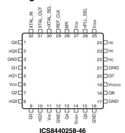
32-Lead VFQFN 5mm x 5mm x 0.925mm package body 3.15mm x 3.15mm ePad size
