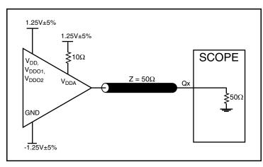
2.5V LVCMOS Output Load Test Circuit
