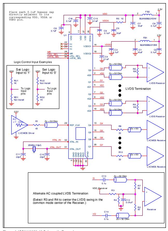
Figure 4. ICS8440258-46 Schematic Example
