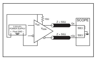
2.5V LVDS Output Load Test Circuit
