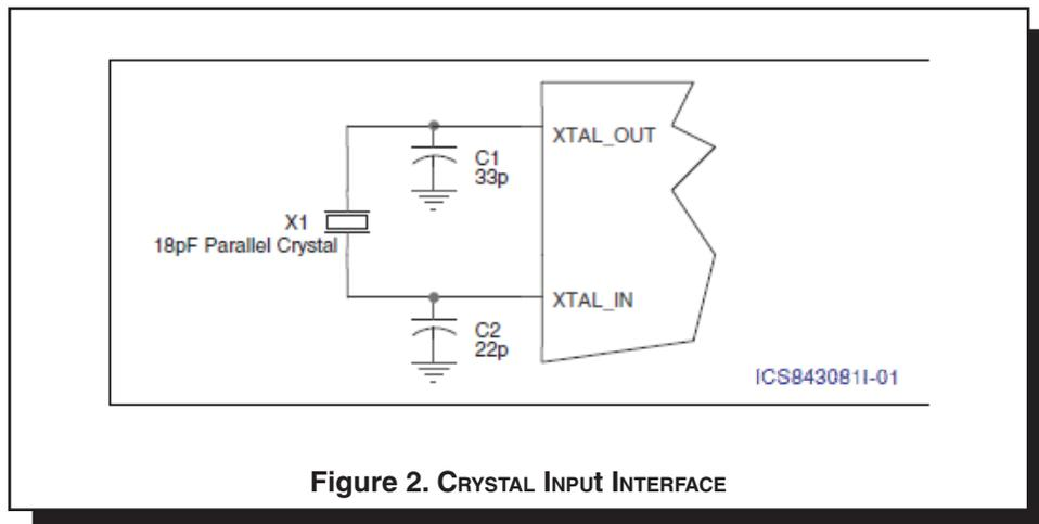
Figure 2. CRYSTAL INPUT INTERFACE
