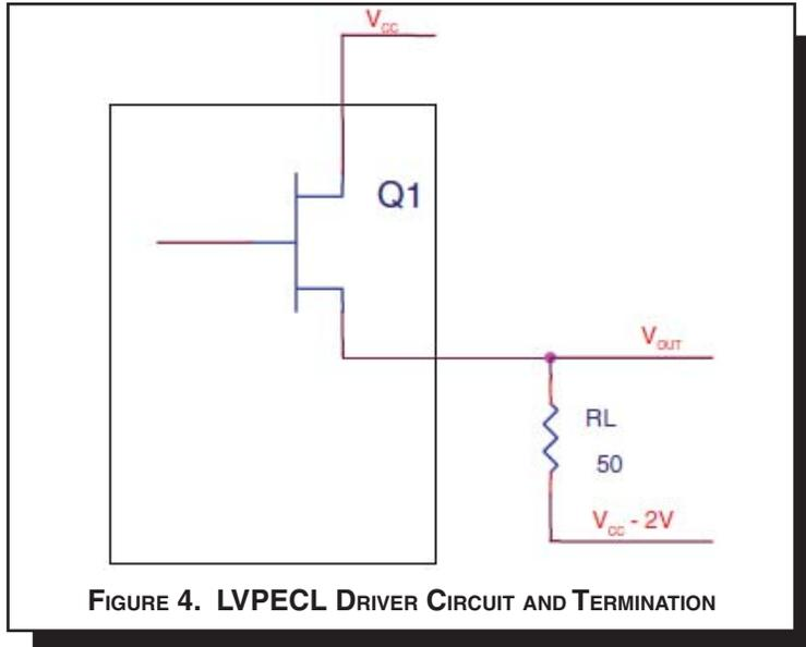
To calculate worst case power dissipation into the load, use the following equations which assume a 50Ω load, and a termination voltage of  $V_{CC} - 2V$ .
