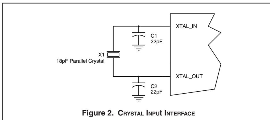
Figure 2. CRYSTAL INPUT INTERFACE
