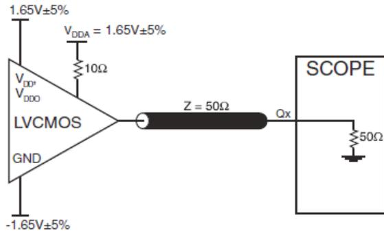
3.3V CORE/3.3V OUTPUT LOAD AC TEST CIRCUIT
