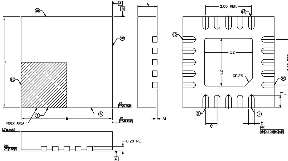
Table 9C. Package Dimensions for 20-Lead VFQFN
