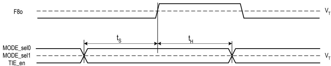
Figure - 15 Input Control Setup and Hold Timing
