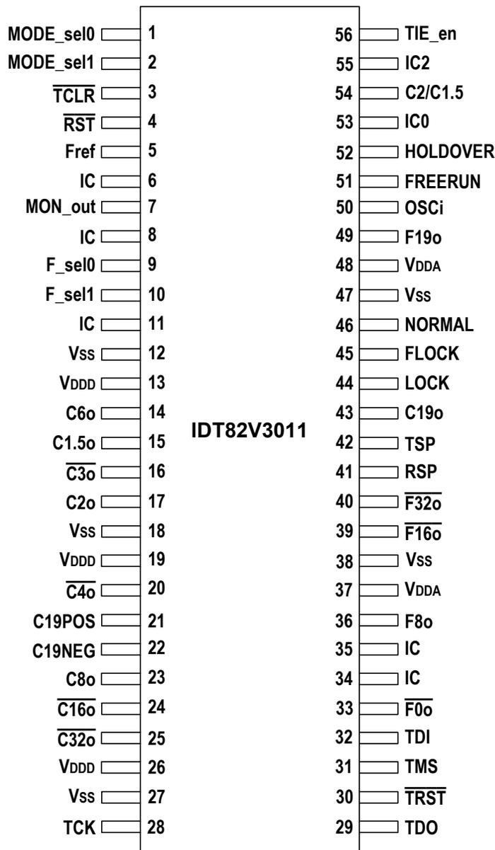
Figure - 1 IDT82V3011 SSOP56 Package Pin Assignment
