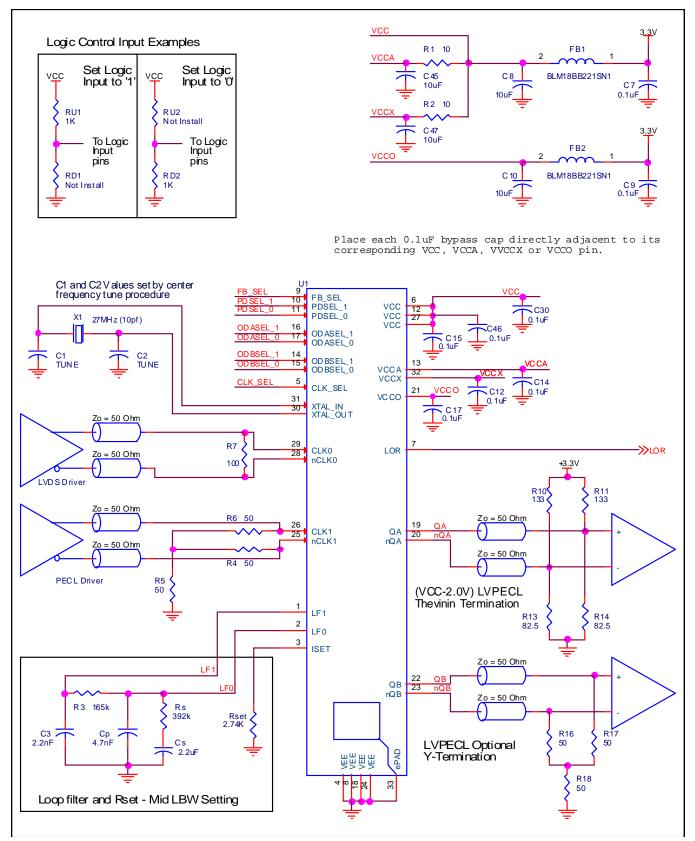
Figure 7. 813N2532I Schematic Example
