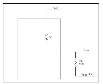
Figure 8. LVPECL Driver Circuit and Termination
