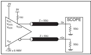
3.3V LVPECL Output Load AC Test Circuit
