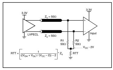
Figure 4A. 3.3V LVPECL Output Termination
