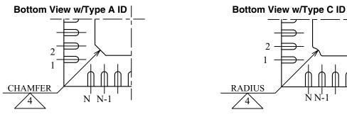
There are 2 methods of indicating pin 1 corner at the back of the VFQFN package:
