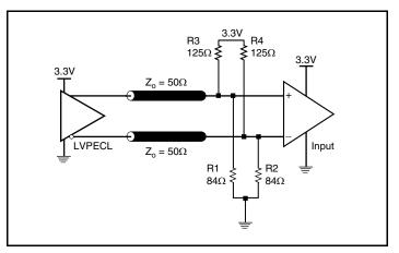
Figure 4B. 3.3V LVPECL Output Termination
