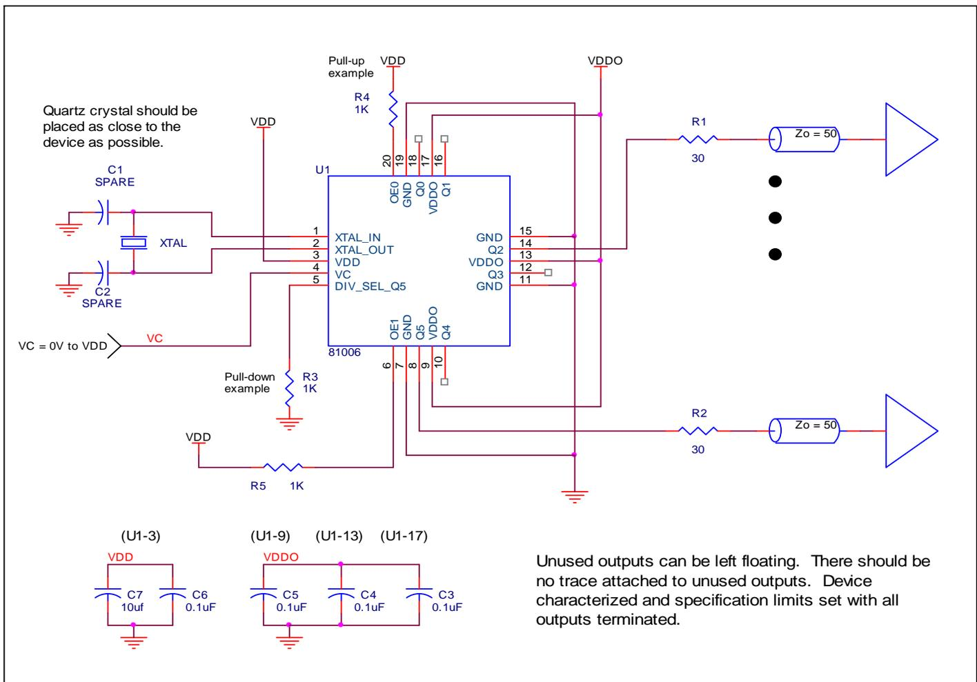
Figure 2. 81006 Schematic Example
