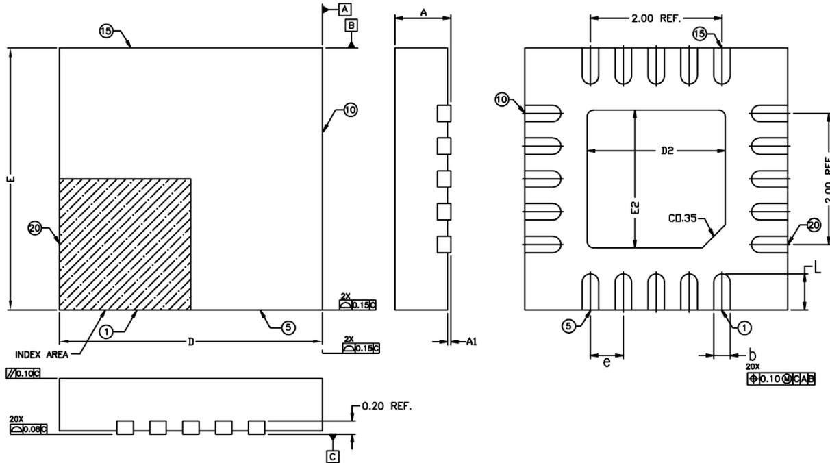
Table 8. Package Dimensions for 20-Lead VFQFN
