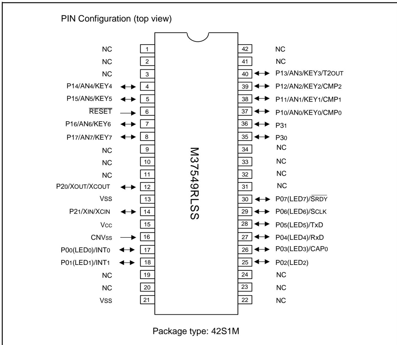
Fig 2. Pin configuration (42S1M type)
