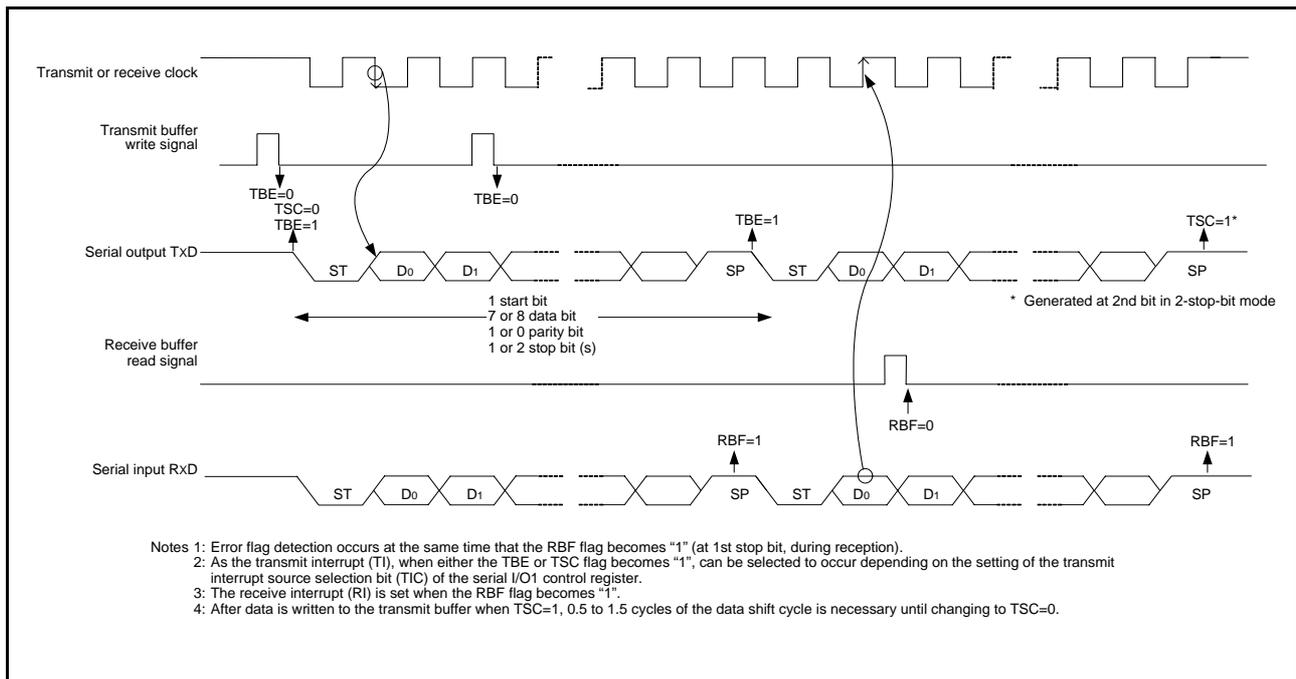
**Fig 49. Operation of UART serial I/O function**
