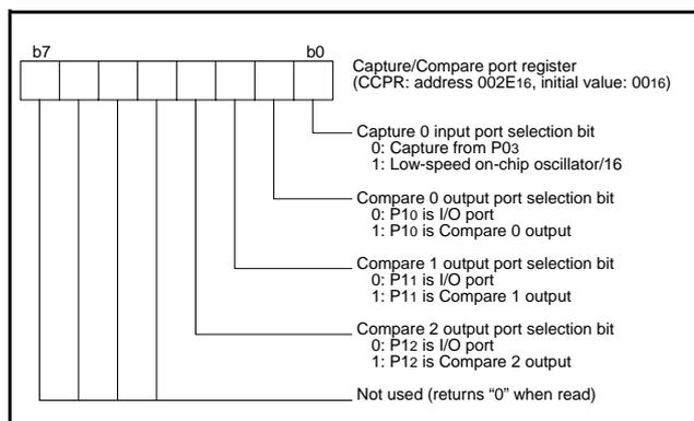
Fig 33. Structure of capture/compare port register
