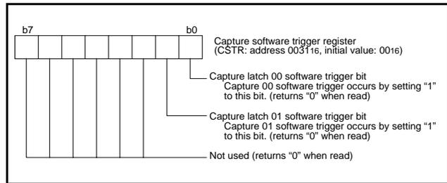
Fig 41. Structure of capture software trigger register
