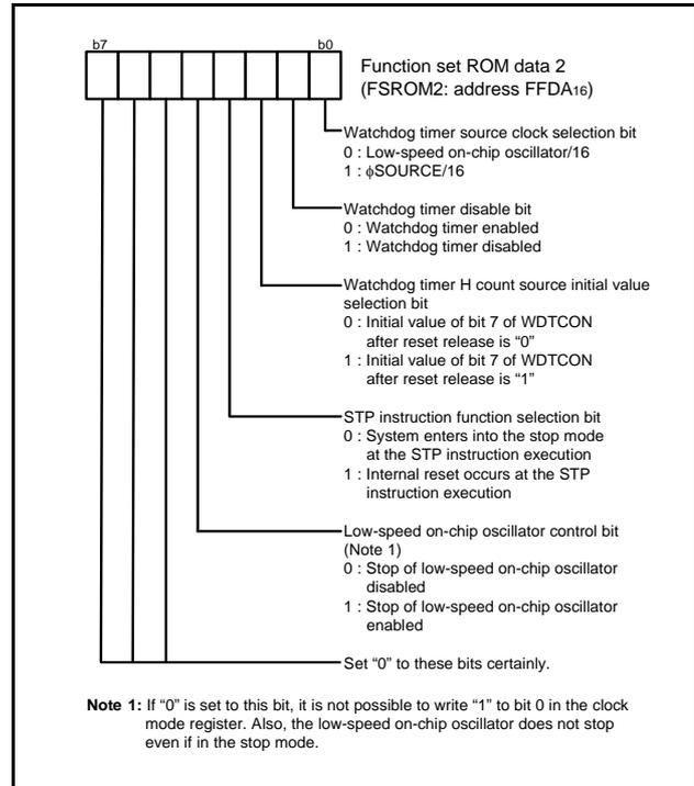
Fig 54. Structure of Function set ROM data 2
