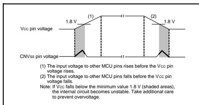
Fig 82. Timing Diagram (bold-lined periods are applicable)
