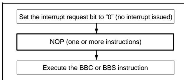
Fig 91. Sequence of check of interrupt request bit
