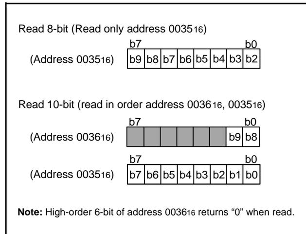
Fig 52. Structure of AD conversion register
