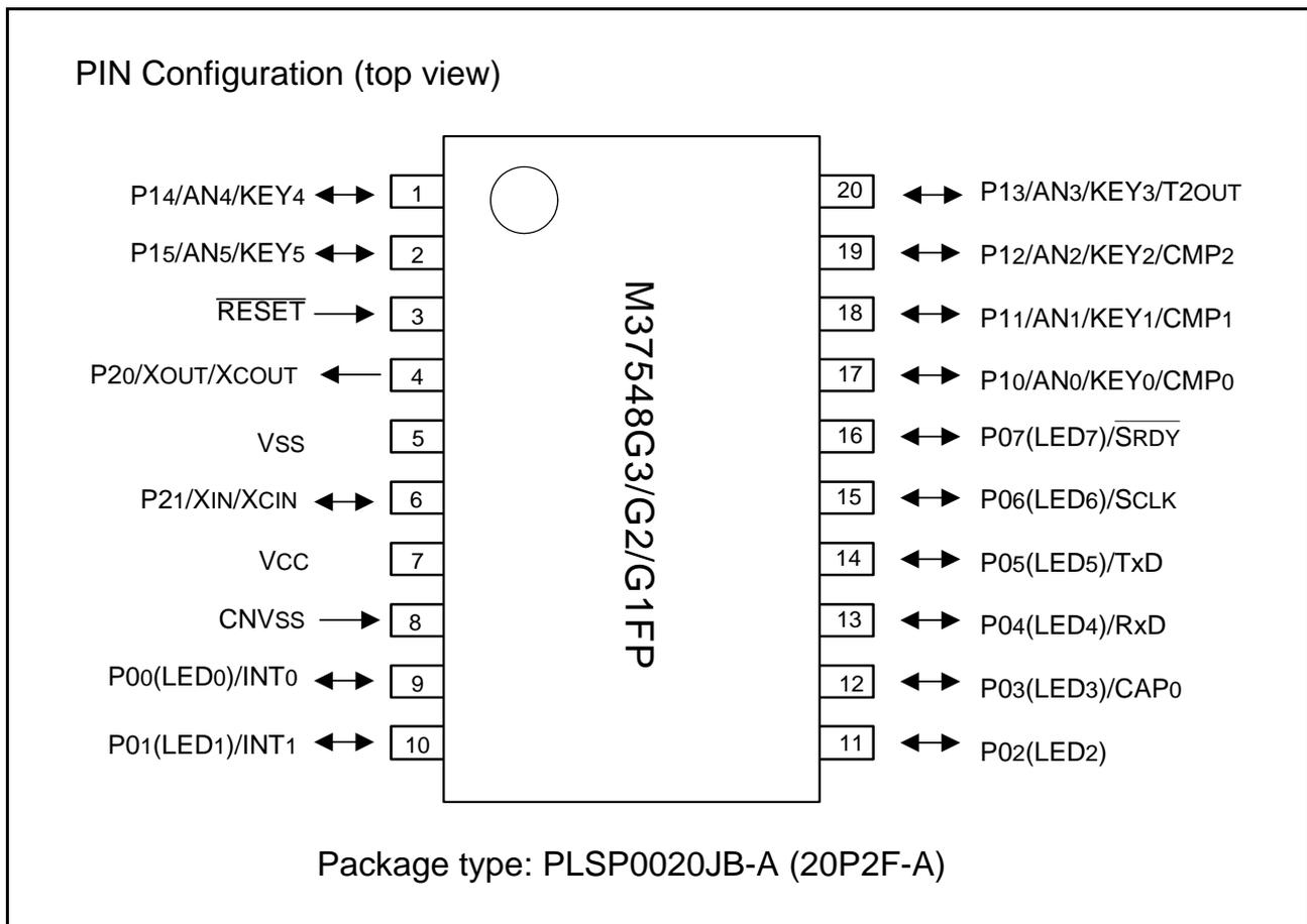
Fig 1. Pin configuration (PLSP0020JB-A type)
