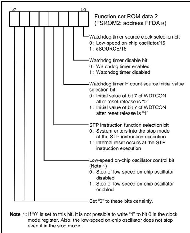
Fig 12. Structure of Function set ROM data 2
