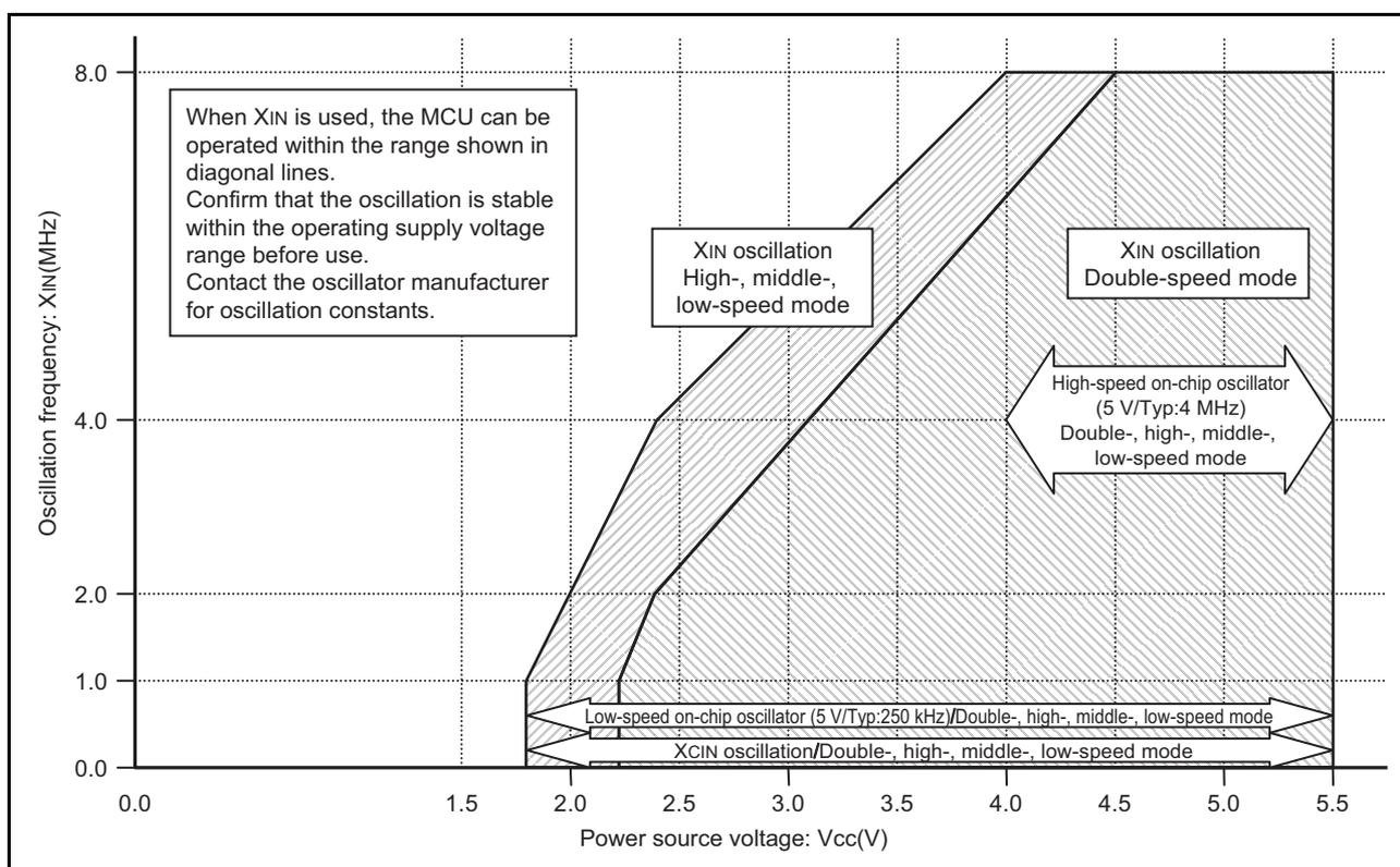
**Fig 83. Power source voltage and oscillation frequency**
