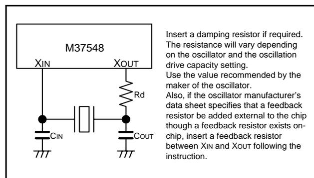
Fig 62. External circuit of ceramic resonator
