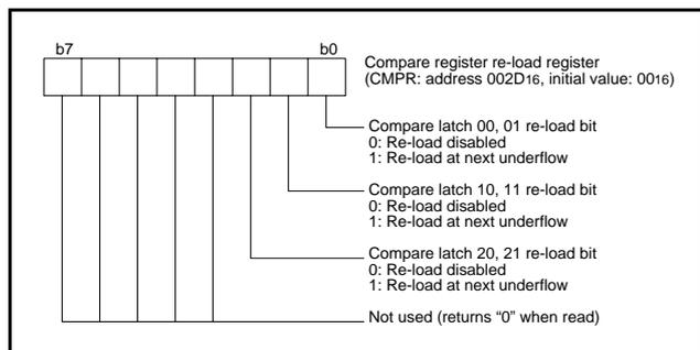
Fig 32. Structure of compare register re-load register
