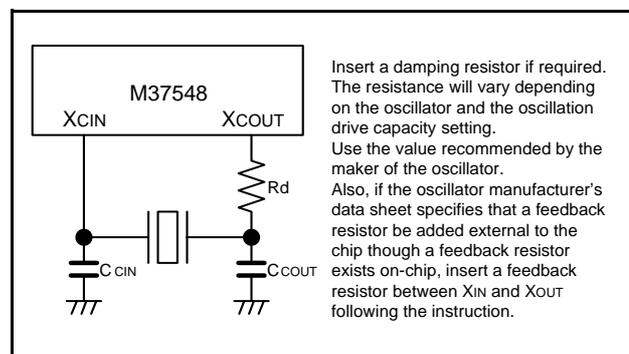
Fig 63. External circuit of 32 kHz quartz-crystal oscillator
