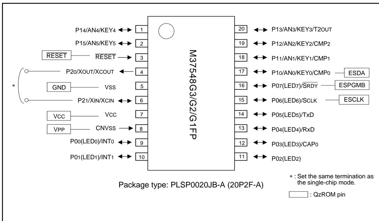
**Fig 70. Pin connection diagram (M37548G3/G2/G1FP)**
