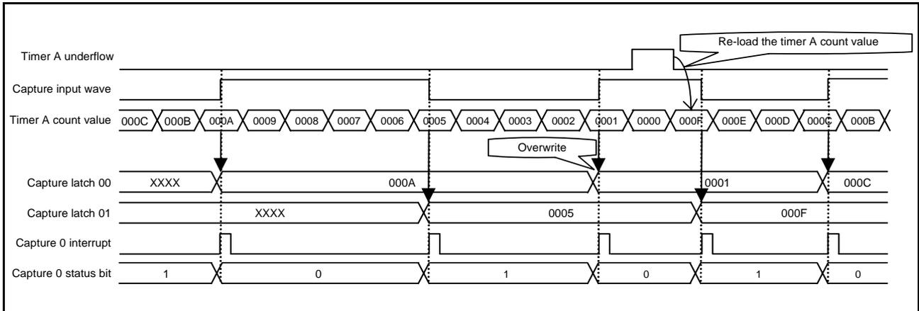
Fig 45. Capture input waveform (capture interrupt edge selection bit = "rising and falling edge")
