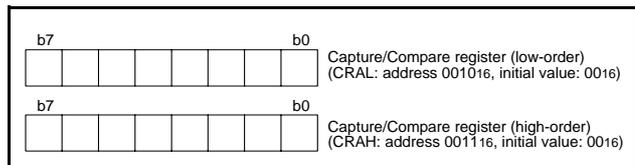
Fig 30. Structure of capture/compare register
