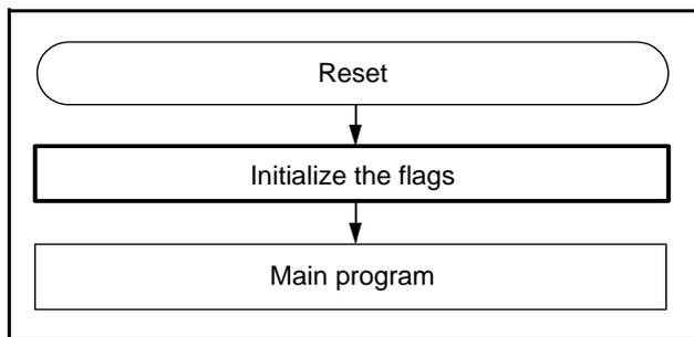
Fig. 87 Initialization of processor status register flags
