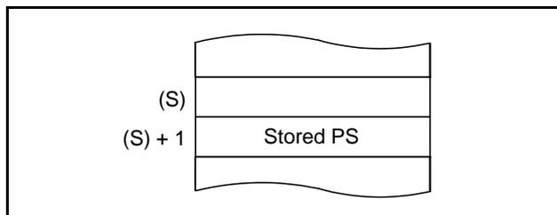
Fig 88. Stack memory contents after PHP instruction execution
