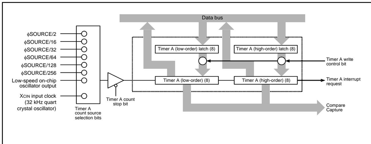
Fig 29. Block diagram of timer A
