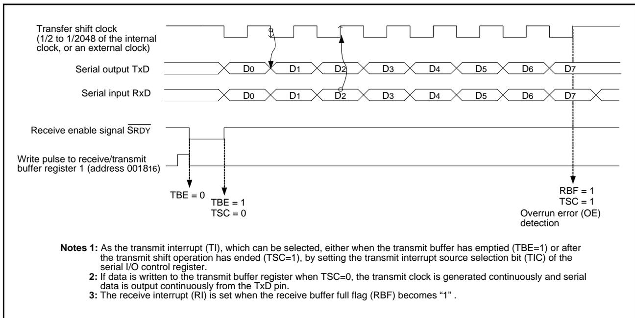
**Fig 47. Operation of clock synchronous serial I/O function**
