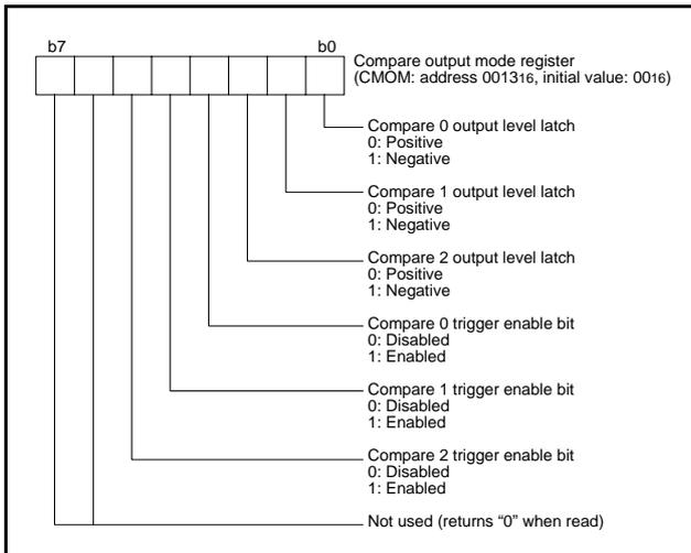
Fig 34. Structure of compare output mode register
