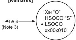
XIN, HSOCO, LSOCO, and respective oscillation and stop status in each mode are shown. The symbol (•) indicates  $\phi$ SOURCE (oscillation) selected by the clock selection bits. "O" indicates oscillation and "S" indicates stopping. The values such as "xx00x010" indicate the values (binary) of the clock mode register in the mode. The arrow (bx) indicates a bit in the clock mode register, showing a transition by changing the bit values.
