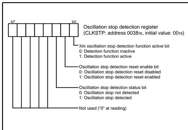
Fig 68. Structure of oscillation stop detection register
