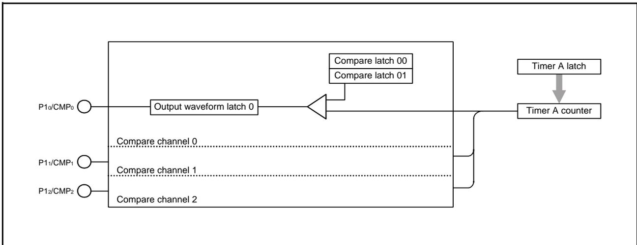
Fig 37. Block diagram of compare output circuit
