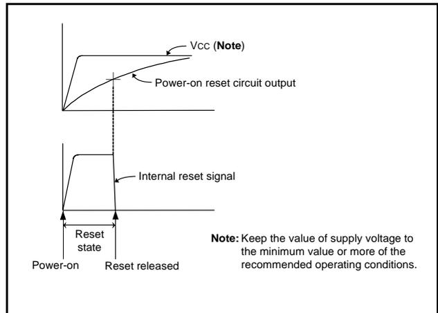
**Fig 57. Operation waveform diagram of power-on reset circuit**
