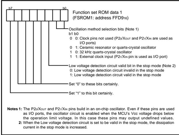
Fig 11. Structure of Function set ROM data 1
