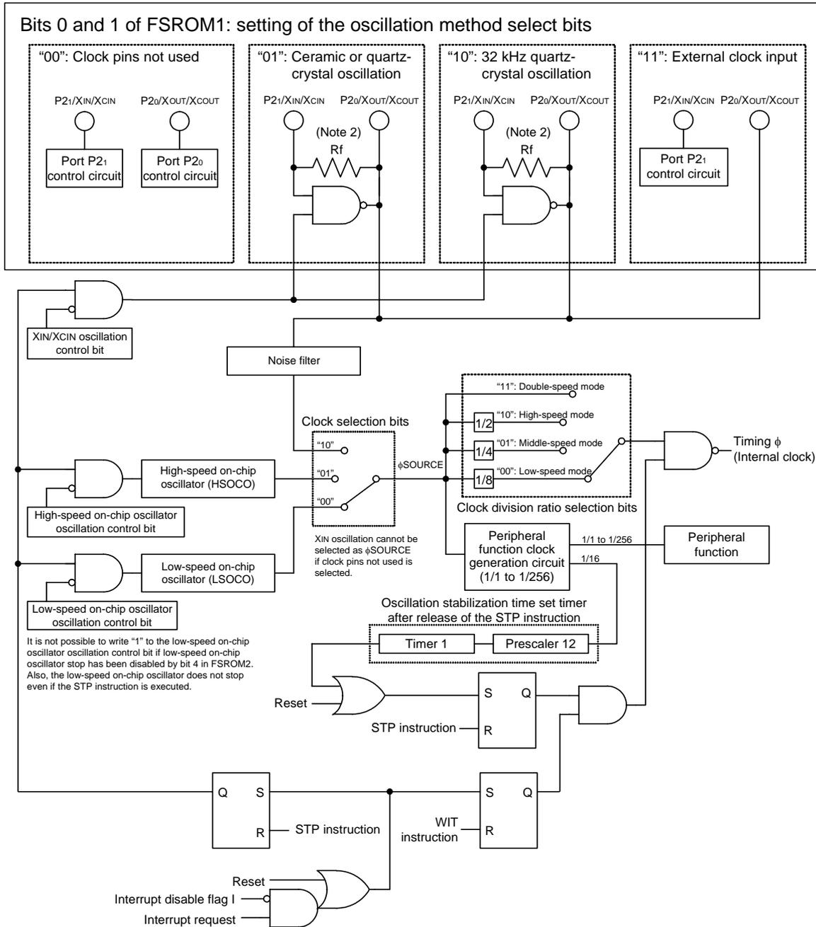
Fig 66. Block diagram of internal clock generating circuit
