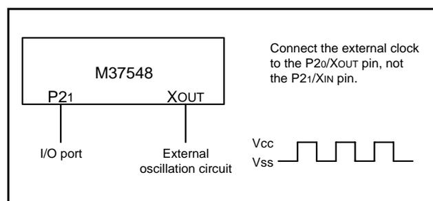
Fig 64. External clock input circuit
