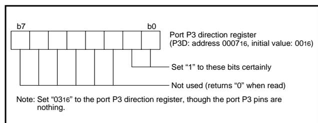
Fig 16. Structure of port P3 direction register
