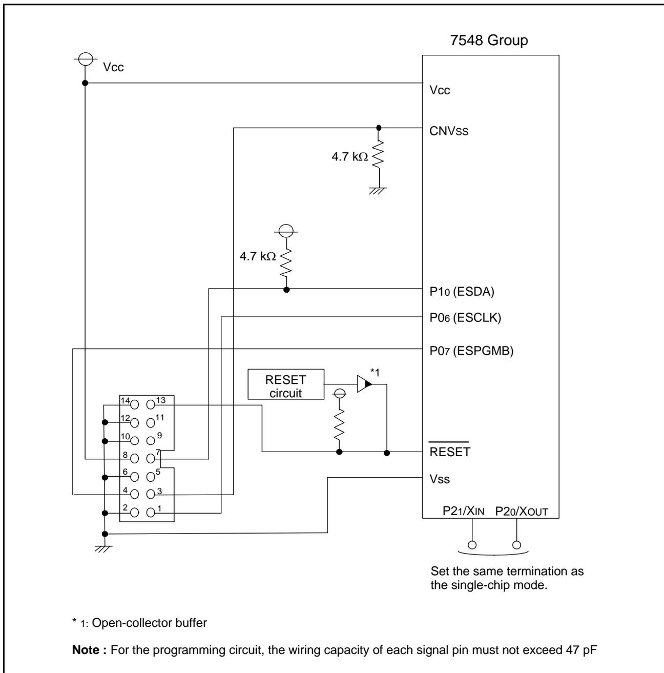
Fig 71. When using E8 programmer, connection example
