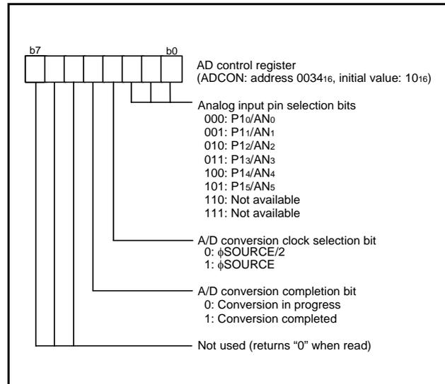
Fig 51. Structure of AD control register
