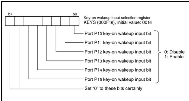
**Fig 25. Structure of key input control register**
