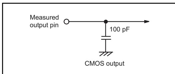
**Fig 85. Switching characteristics measurement circuit diagram**
