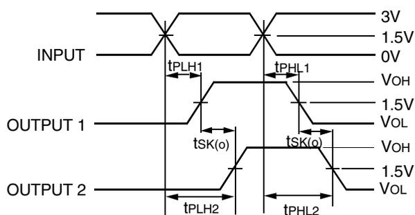
$$t_{SK}(O) = |t_{PLH2} - t_{PLH1}| \text{ or } |t_{PHL2} - t_{PHL1}|$$
