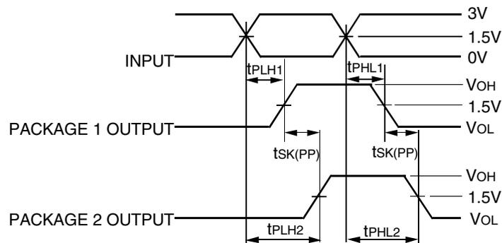
$$t_{SK}(PP) = |t_{PLH2} - t_{PLH1}| \text{ or } |t_{PHL2} - t_{PHL1}|$$
