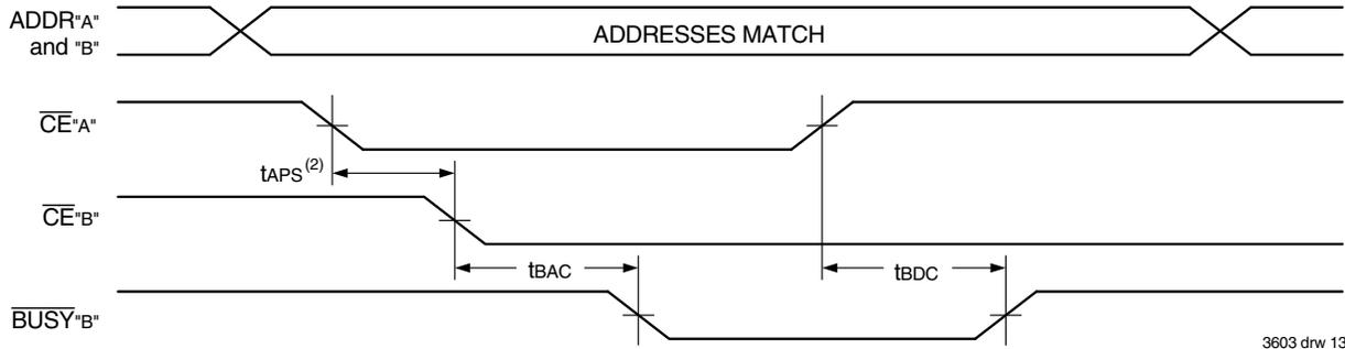
Waveform of **BUSY** Arbitration Cycle Controlled by Address Match Timing ( $M/\bar{S} = V_{IH}$ )<sup>(1)</sup>
