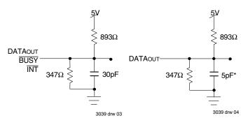
Figure 1. AC Output Test Load
