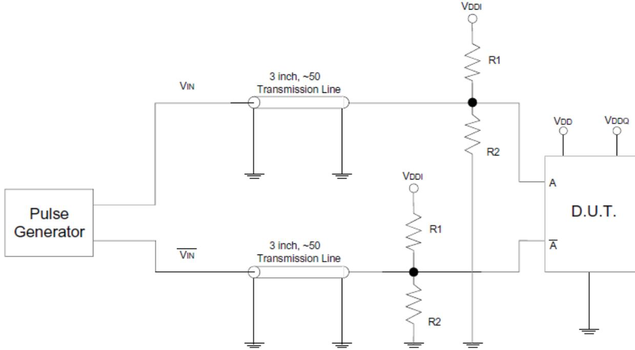
Test Circuit for Differential Input<sup>(1)</sup>
