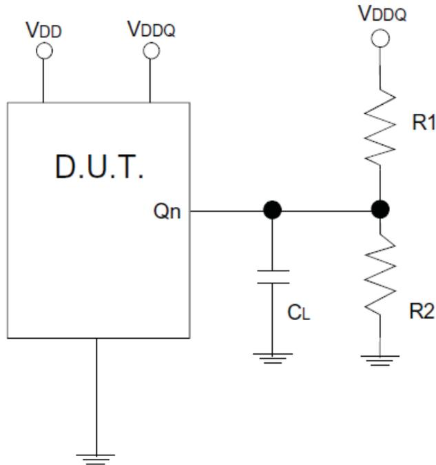
*Test Circuit for SDR Outputs*
