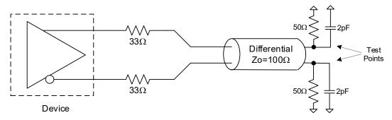
Figure 4. LVDS Test Load
