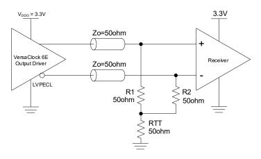
Figure 14. 2.5V LVPECL Output Termination (1)
