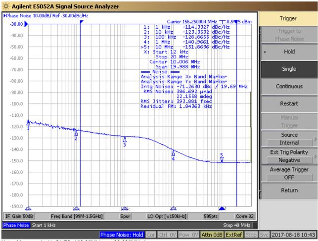
Note: Measured with OUT2=156.25MHz on, 39.625MHz input.
