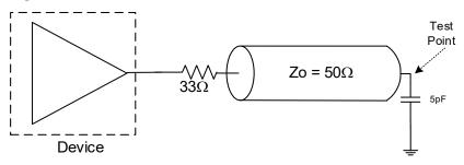
Figure 3. HCSL/LPHCSL Test Load
