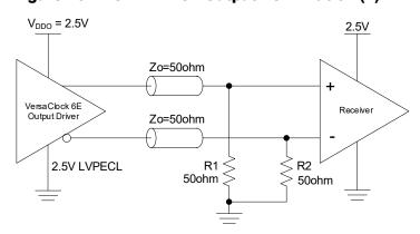
Figure 16. 2.5V LVPECL Output Termination (3)
