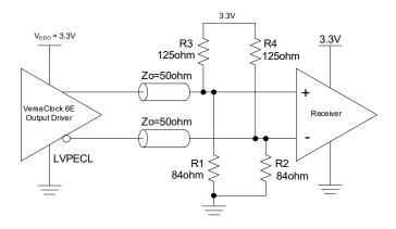
Figure 15. 2.5V LVPECL Output Termination (2)
