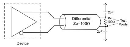
Figure 5. LVPECL Test Load
