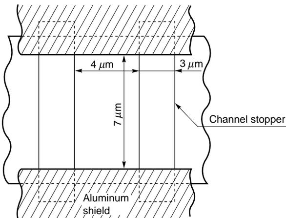
**PHOTOCELL ARRAY STRUCTURE DIAGRAM (Line spacing)**
