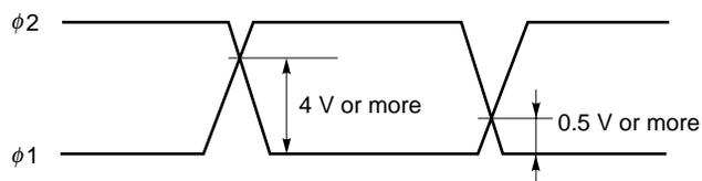
**Remark** Adjust cross points of φ1 and φ2 with input resistance of each pin.
