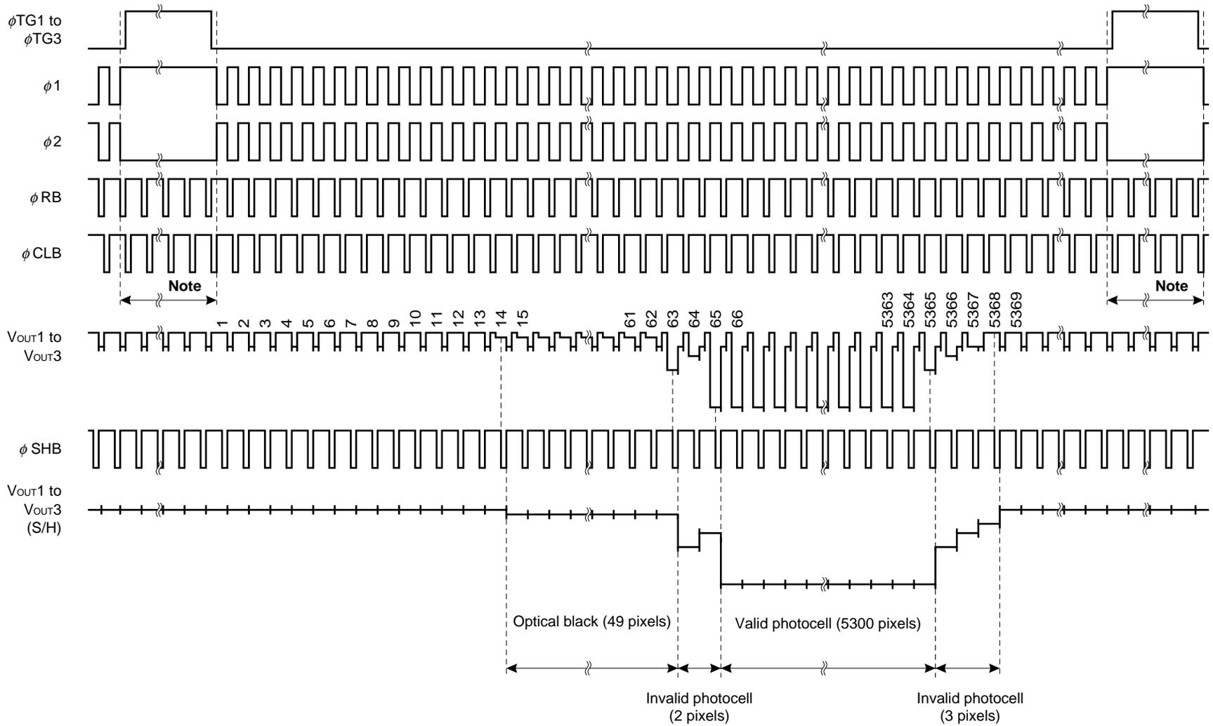
**Note** Input the  $\phi RB$  and  $\phi CLB$  pulses continuously during this period. And also input the  $\phi SHB$  pulse when the on-chip sample and hold function is used.
