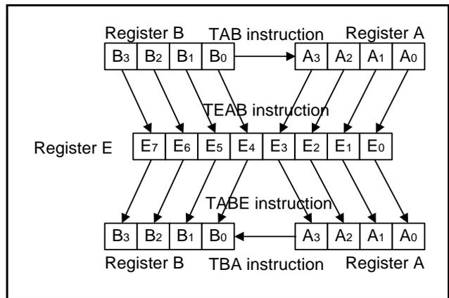
**Fig 14. Registers A, B and register E**
