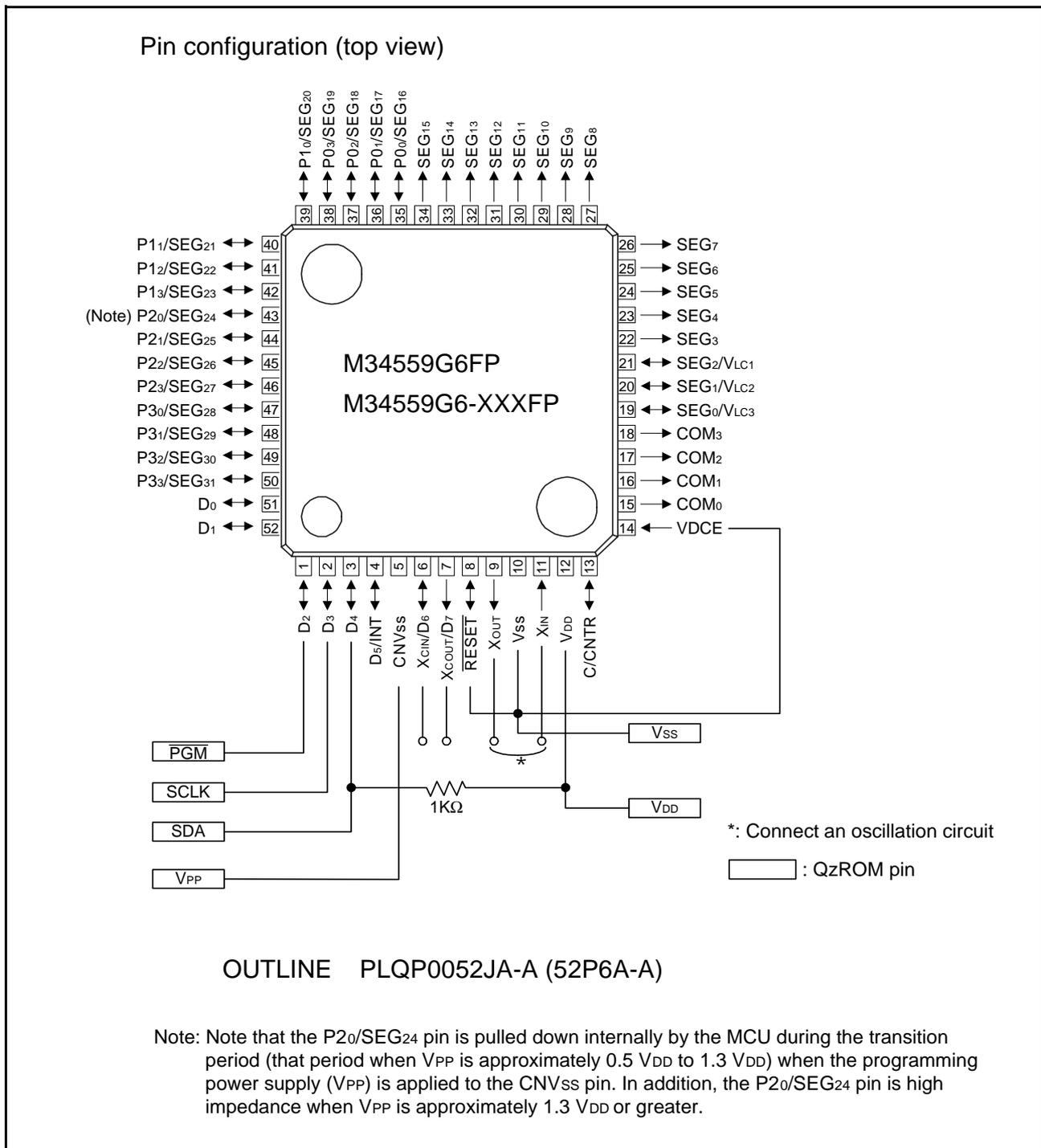
Fig 66. Pin connection diagram
