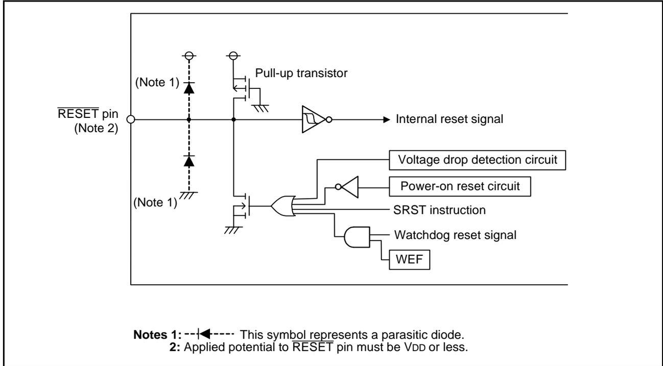
**Fig 48. Structure of RESET pin and its peripherals**
