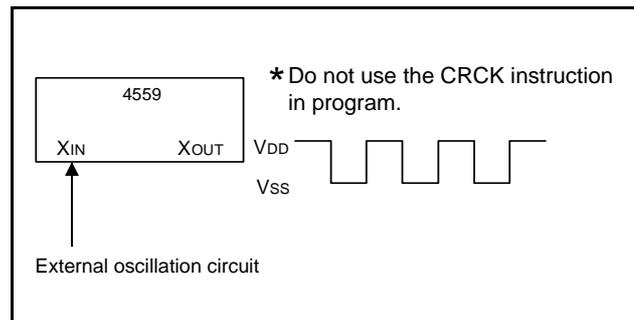
**Fig 64. External clock input circuit**
