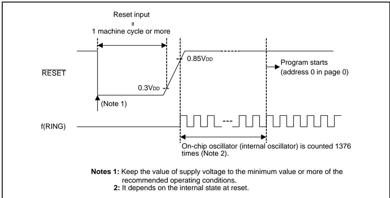
**Fig 49. RESET pin input waveform and reset release timing**
