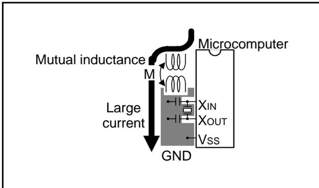
**Fig 78. Wiring for a large current signal line**
