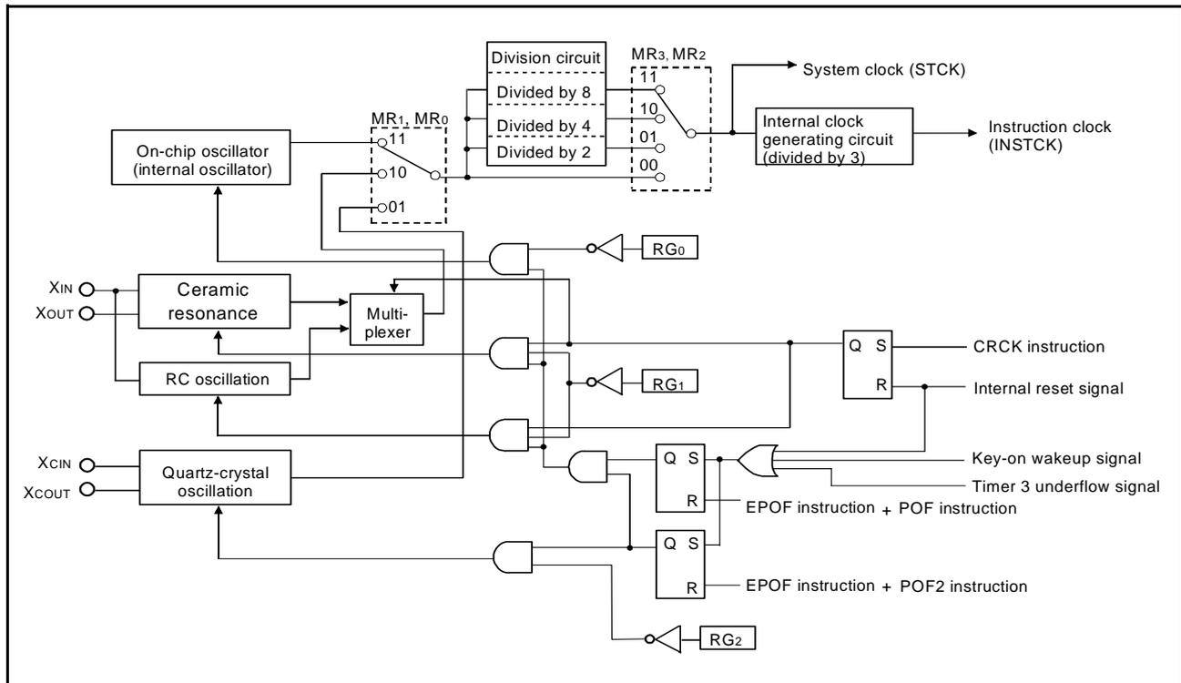
Fig 59. Clock control circuit structure
