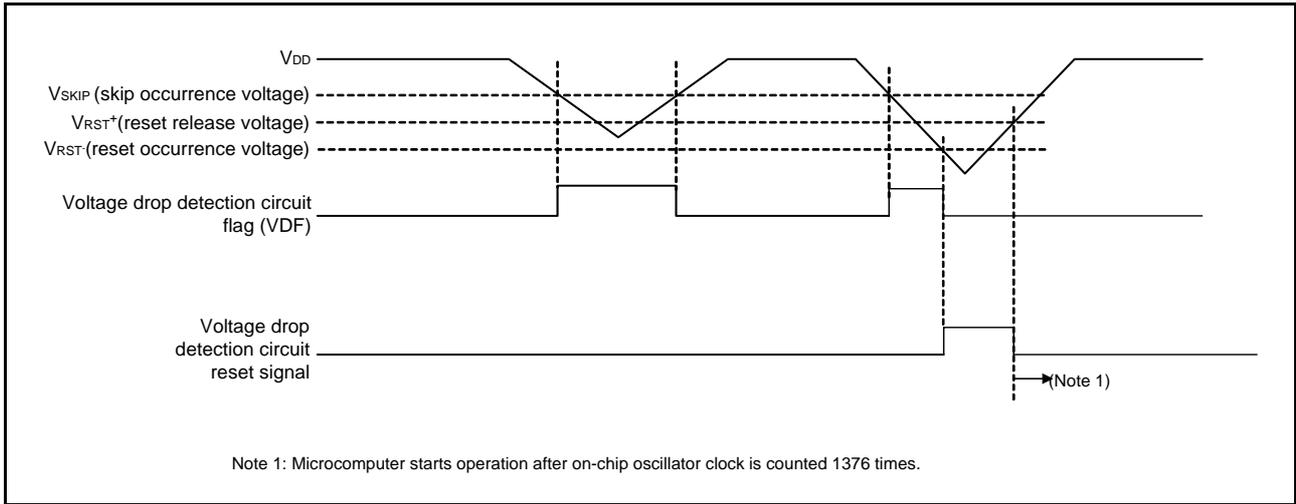
**Fig 54. Voltage drop detection circuit operation waveform**
