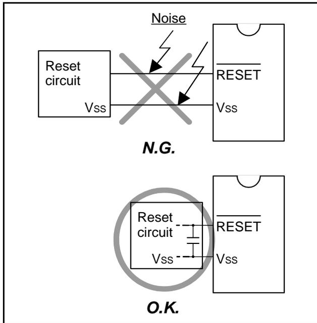
**Fig 74. Wiring for the RESET input pin**
