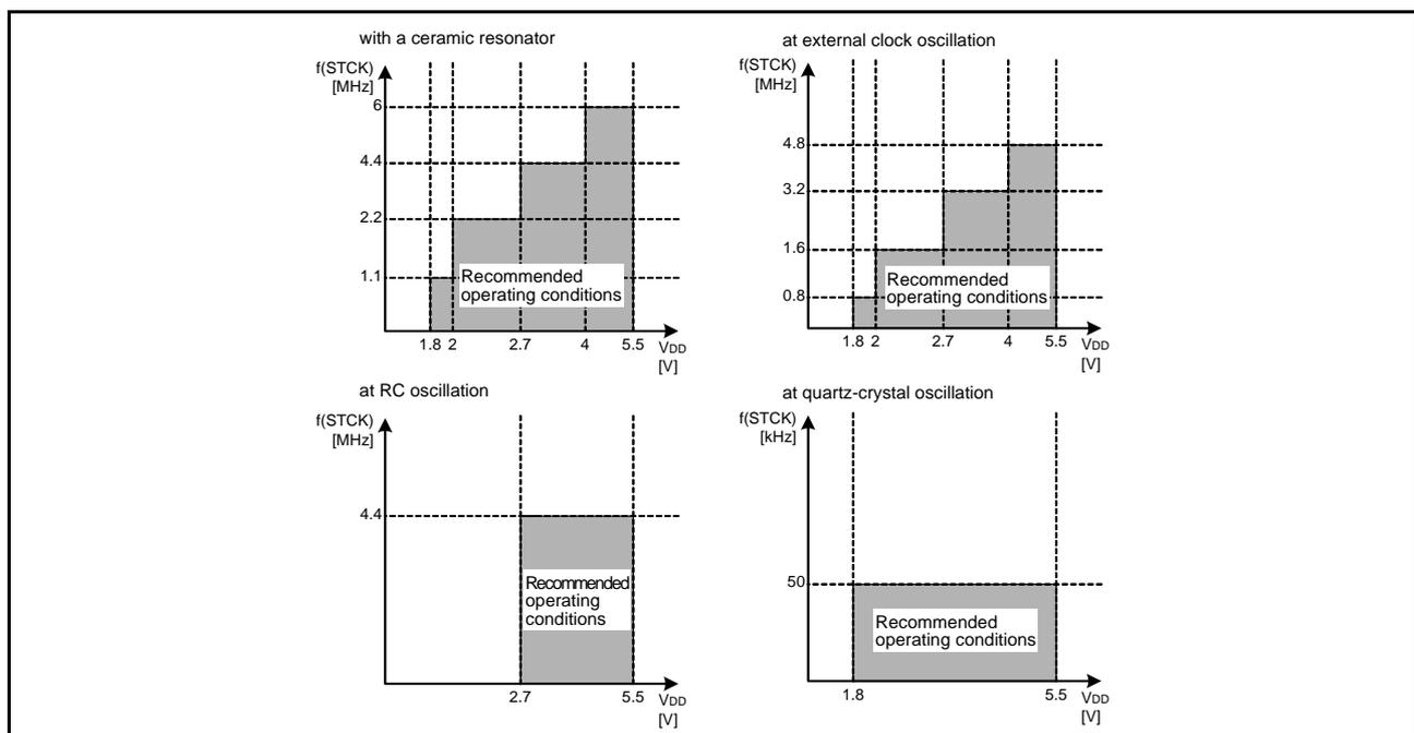
**Fig 82. System clock (STCK) operating condition map**
