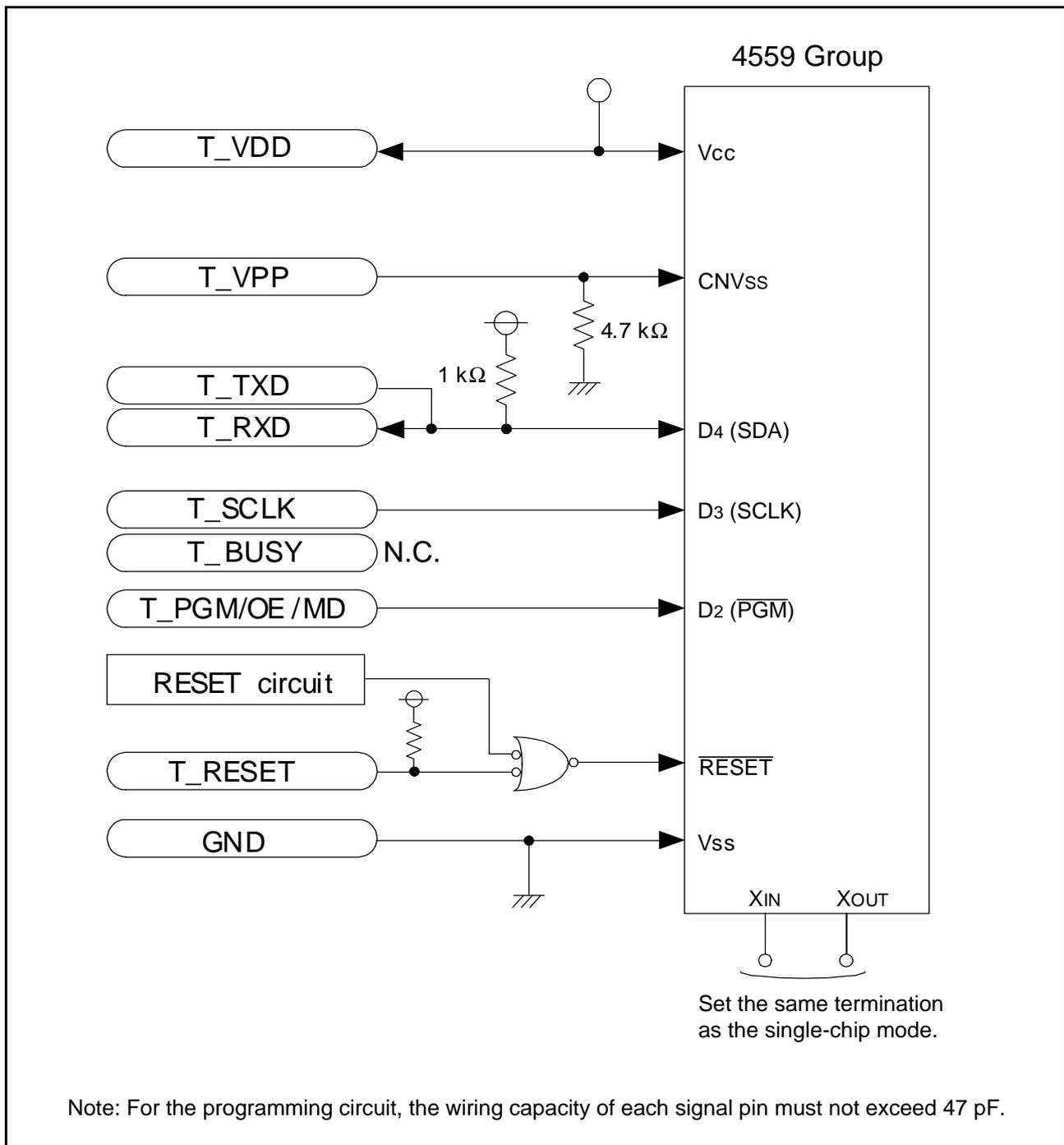
Fig 67. When using programmer of Suisai Electronics System Co., LTD, connection example
