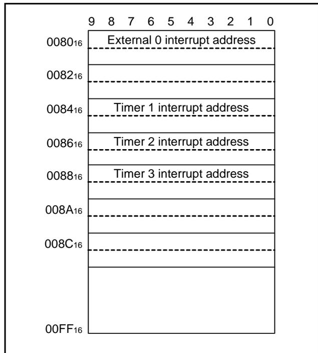
**Fig 22. Page 1 (addresses 0080<sub>16</sub> to 00FF<sub>16</sub>) structure**
