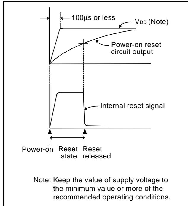
Fig 50. Power-on reset operation
