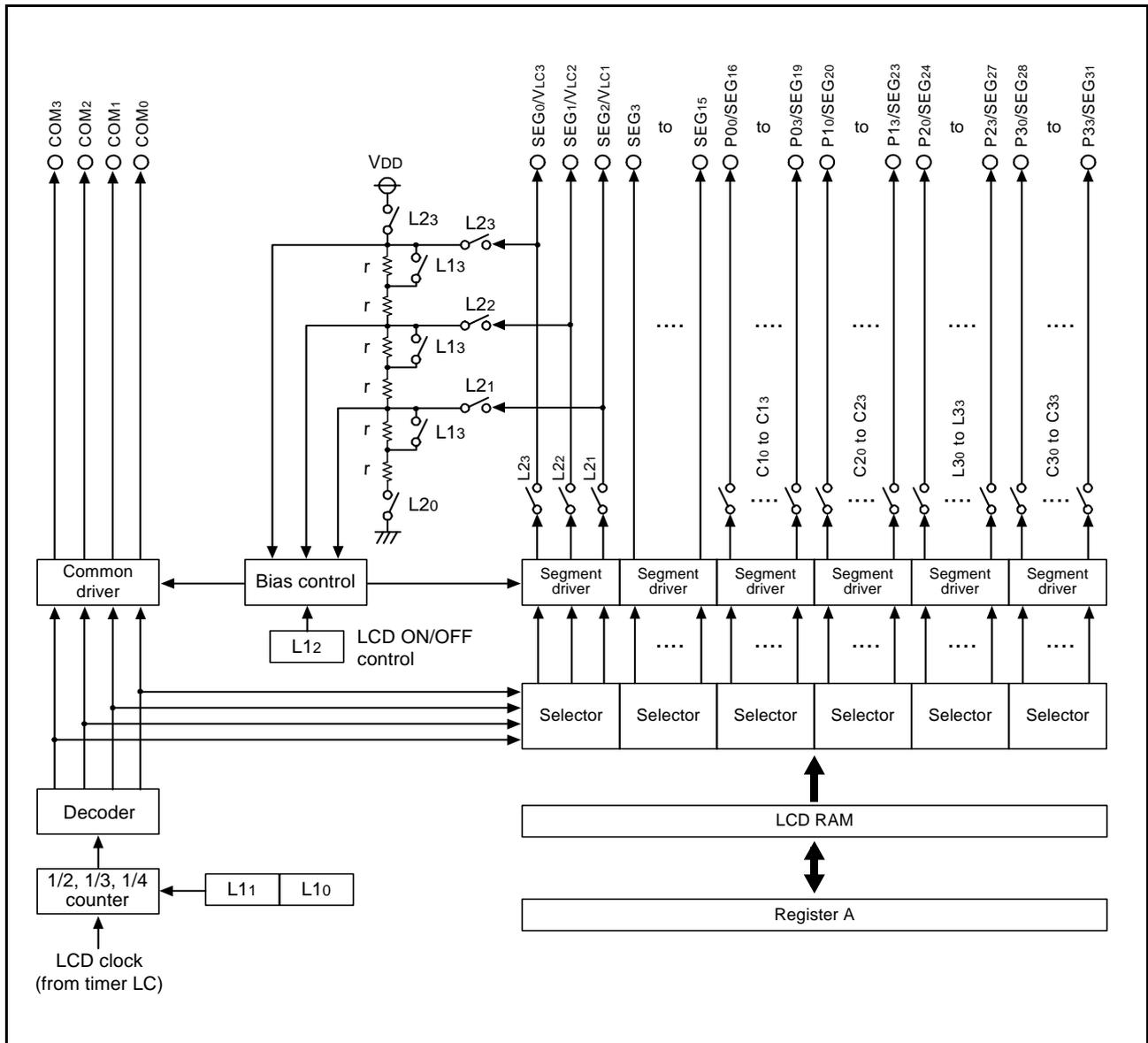
**Fig 43. LCD controller/driver**
