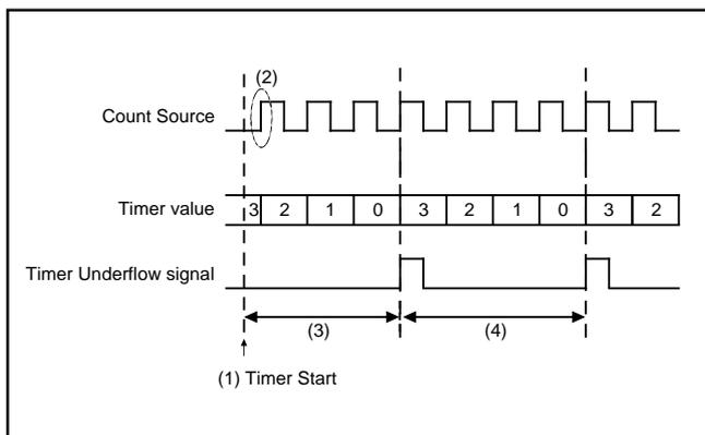
**Fig. 29 Timer count start timing and count time when operation starts (Prescaler, Timer 1, Timer 2 and Timer 3)**
