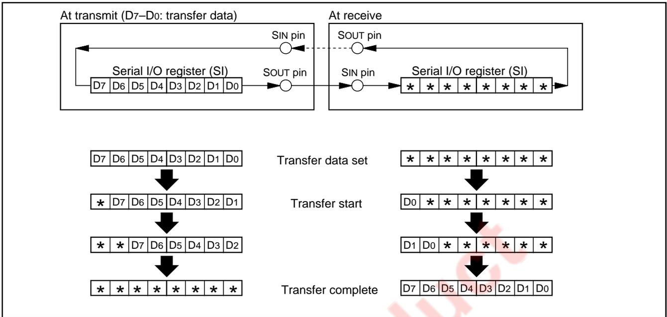
Fig. 43 Serial I/O register state when transferring
