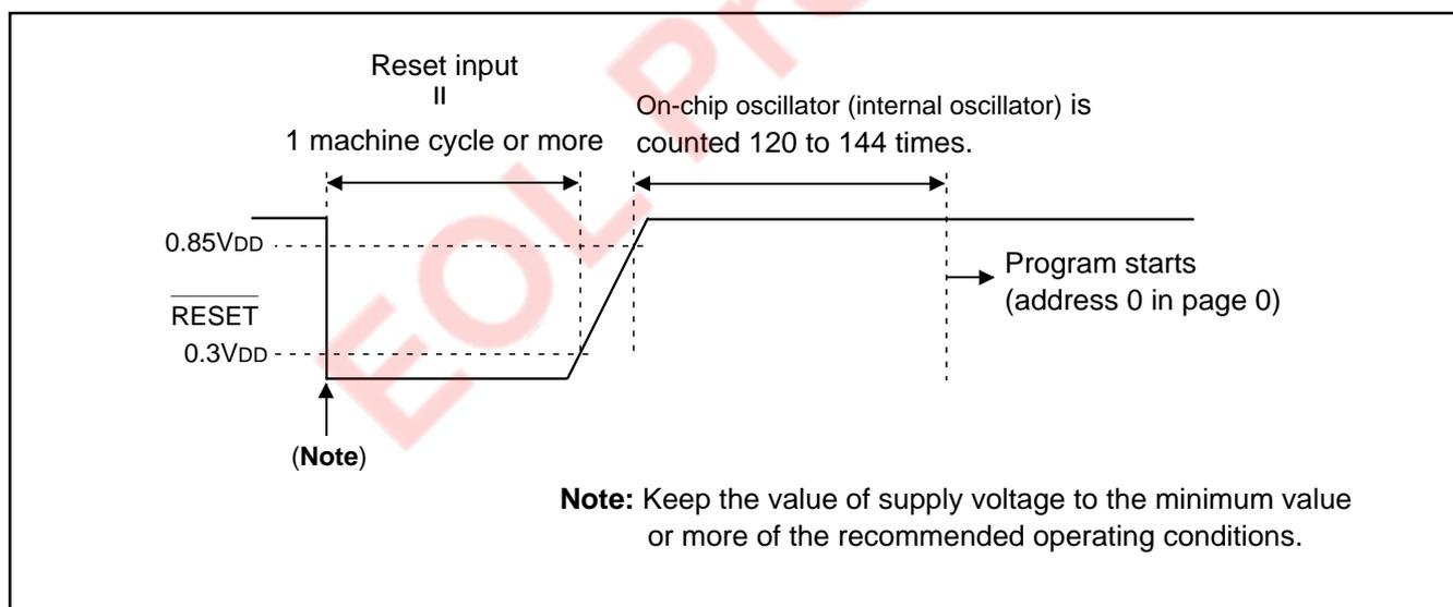
Fig. 47  $\overline{\text{RESET}}$  pin input waveform and reset operation
