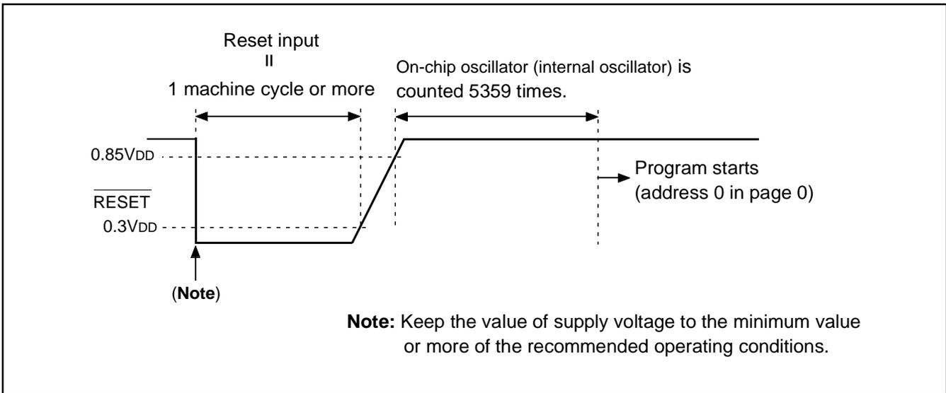
Fig. 34  $\overline{\text{RESET}}$  pin input waveform and reset operation
