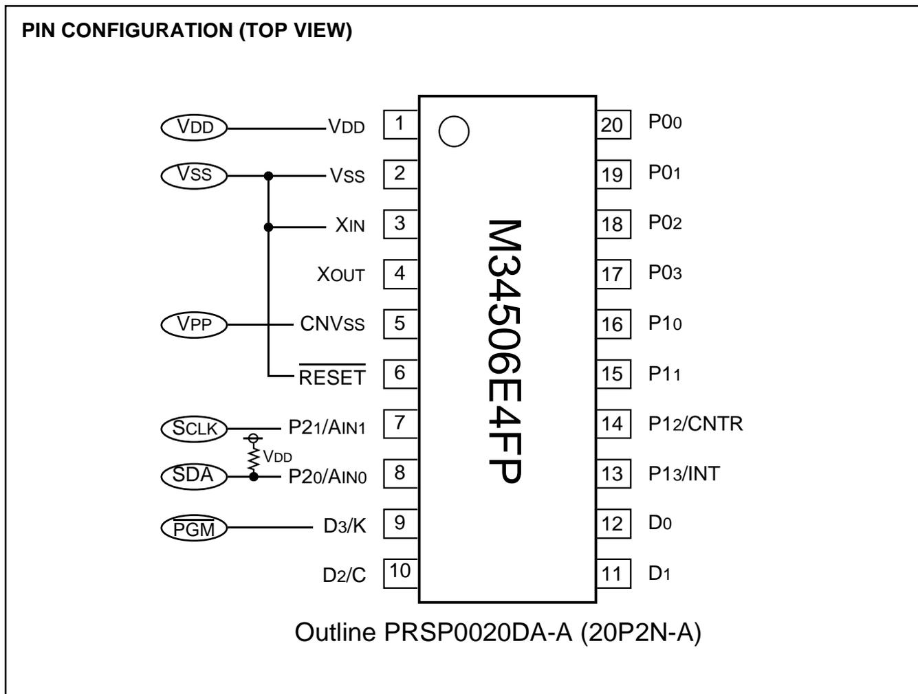
Fig. 54 Pin configuration of built-in PROM version
