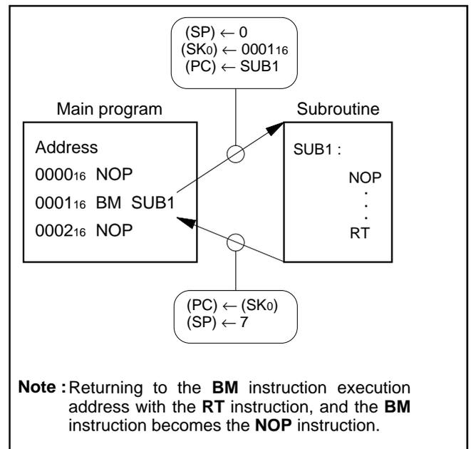
Fig. 6 Example of operation at subroutine call
