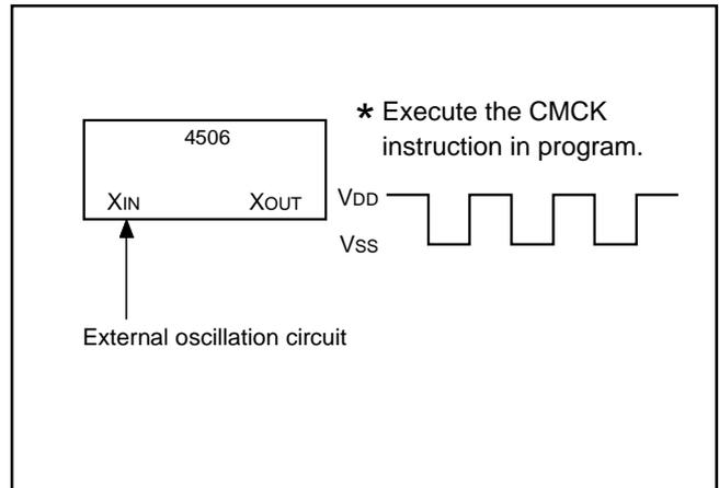
Fig. 45 External clock input circuit
