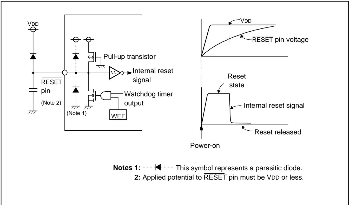
Fig. 35 Structure of reset pin and its peripherals, and power-on reset operation
