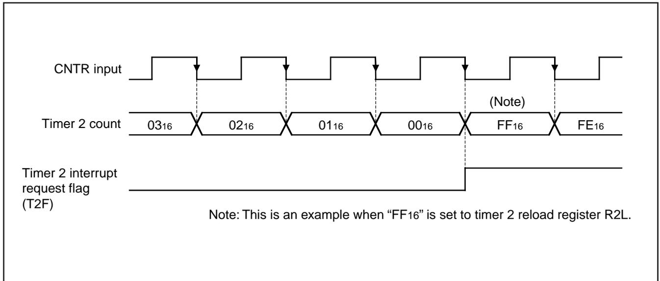
Fig. 23 Count timing diagram at CNTR input
