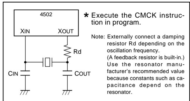
Fig. 45 Ceramic resonator external circuit
