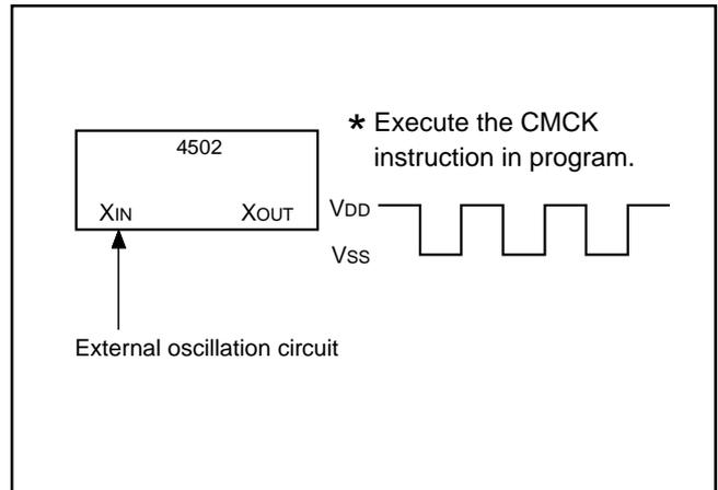
Fig. 47 External clock input circuit
