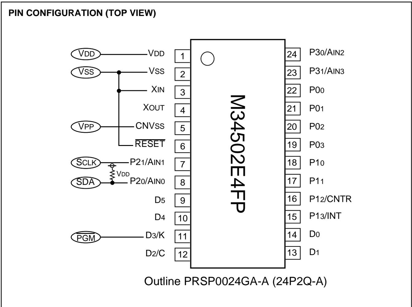
Fig. 56 Pin configuration of built-in PROM version
