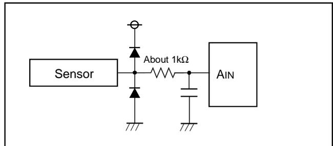
Fig. 54 Analog input external circuit example-2
