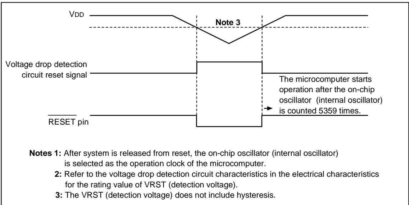
Fig. 38 Voltage drop detection circuit operation waveform example
