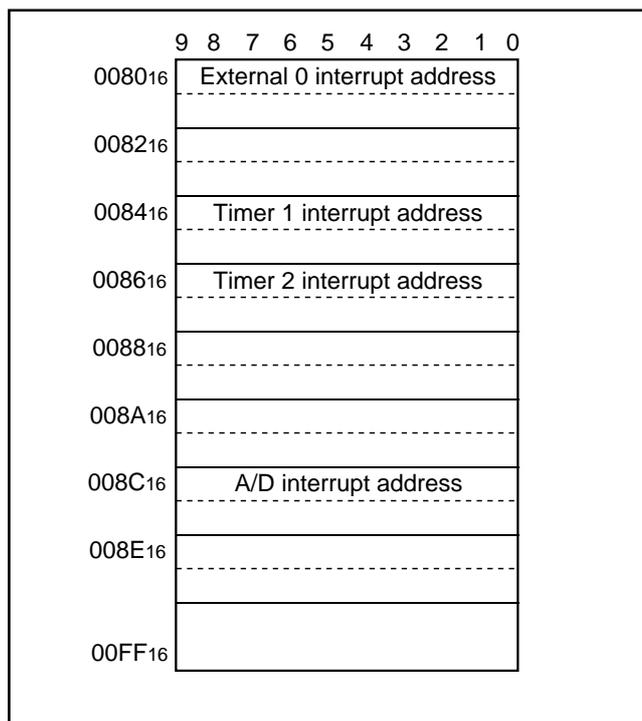
**Fig. 11 Page 1 (addresses 0080<sub>16</sub> to 00FF<sub>16</sub>) structure**
