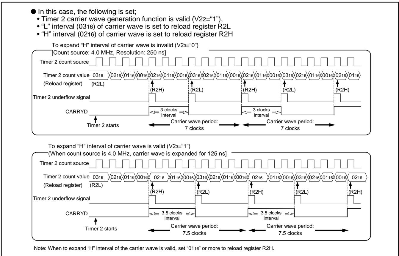
Fig. 16 Carrier wave generation example by timer 2
