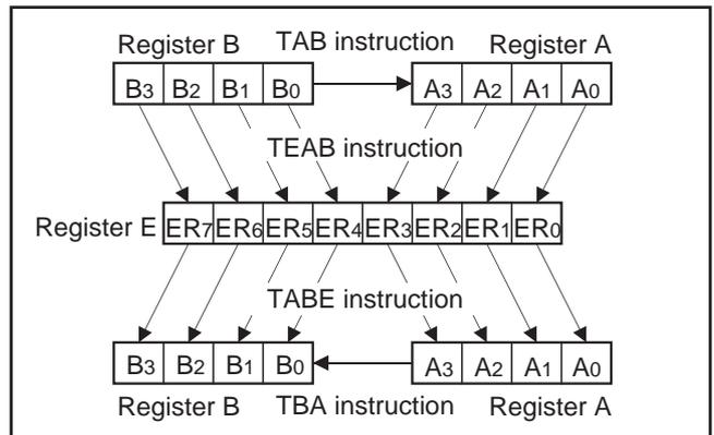
**Fig. 3 Registers A, B and register E**
