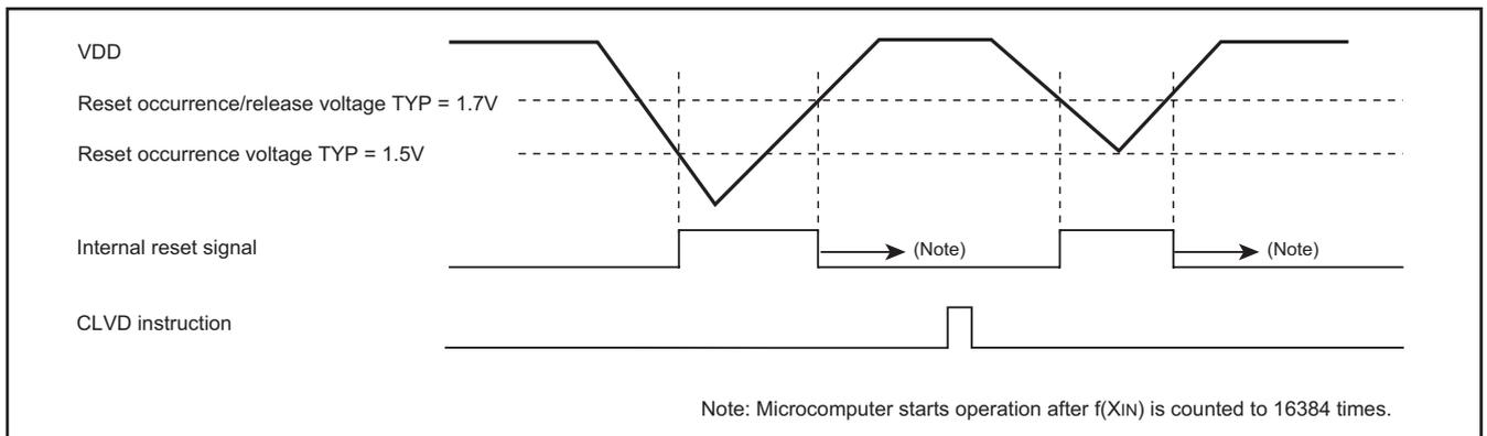
Fig. 22 Voltage drop detection circuit operation waveform
