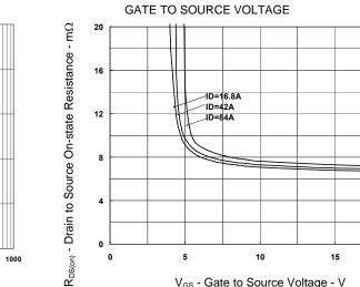
DRAIN TO SOURCE ON-STATE RESISTANCE vs.
