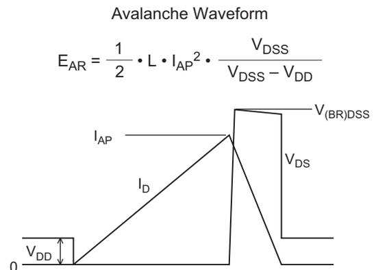
$$E_{AR} = \frac{1}{2} \cdot L \cdot I_{AP}^2 \cdot \frac{V_{DSS}}{V_{DSS} - V_{DD}}$$
