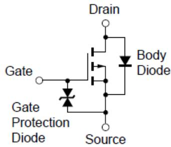
**Remark** The diode connected between the gate and source of the transistor serves as a protector against ESD. When this device actually used, an additional protection circuit is externally required if a voltage exceeding the rated voltage may be applied to this device.
