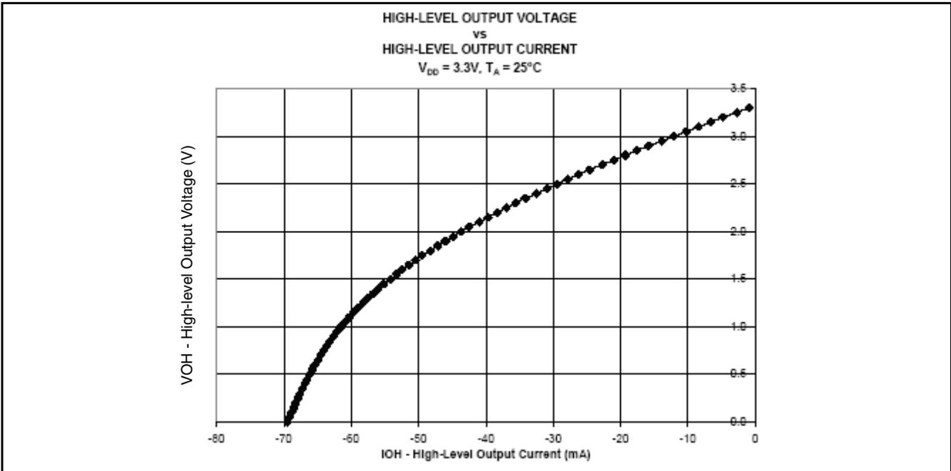
Figure 6. High-level Output Voltage vs. High-level Output Current
