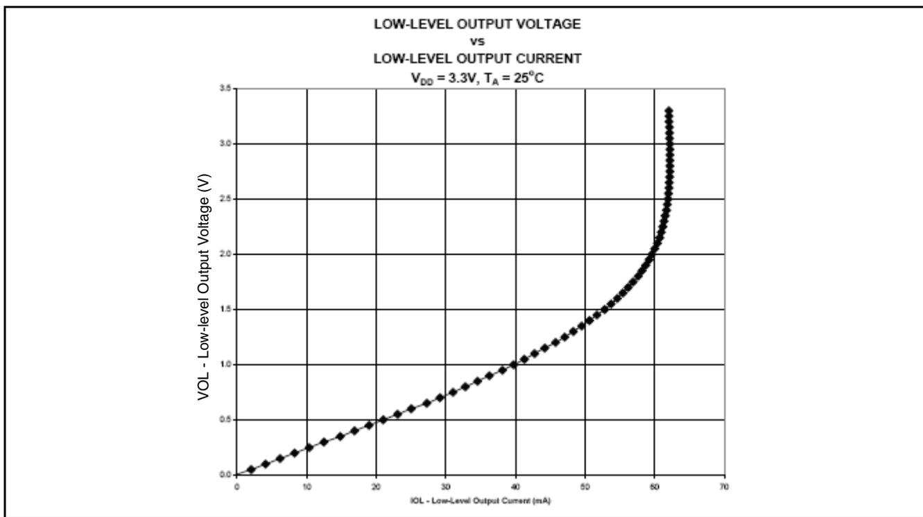
Figure 7. Low-level Output Voltage vs. Low-level Output Current
