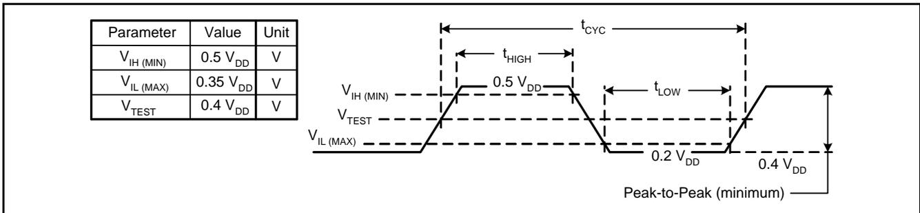
Figure 4. Clock Waveform
