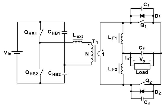
Fig. 1 Simplified circuit diagram of AE's new resonant converter
