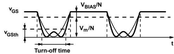
Fig. 14 Improved gate-drive voltage waveform
