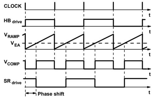
Fig. 11 Key waveforms of the control circuit
