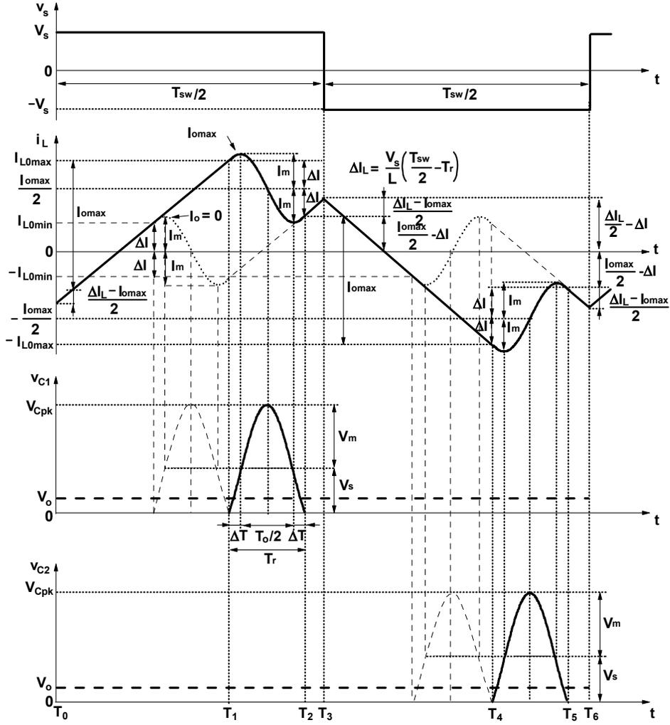
Fig. 5 Key waveforms in Mode I
