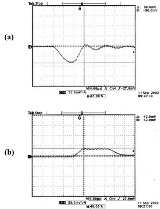
Fig. 17 Output voltage waveform at slow load-current transient (a) 0-75 A and (b) 75-0 A with 10 A/ $\mu$ s current slope ( $V_{in} = 48$  V,  $V_o = 1.3$  V)
