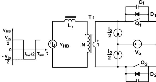
Fig. 2 Equivalent circuit of AE's new resonant converter
