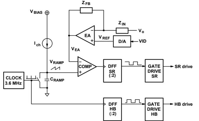
Fig. 10 Functional block diagram of the control circuit
