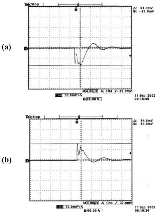
Fig. 16 Output voltage waveform at fast load-current transient (a) 75-100 A and (b) 100-75 A with 100 A/ $\mu$ s current slope ( $V_{in} = 48$  V,  $V_o = 1.3$  V)
