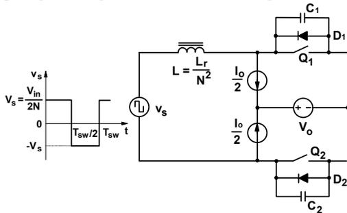
Fig. 3 Simplified equivalent circuit of AE's new resonant converter
