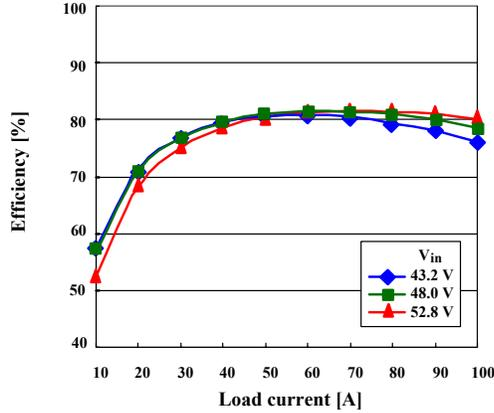
Fig. 15 Efficiency measurements at nominal output voltage  $V_o = 1.3$  V
