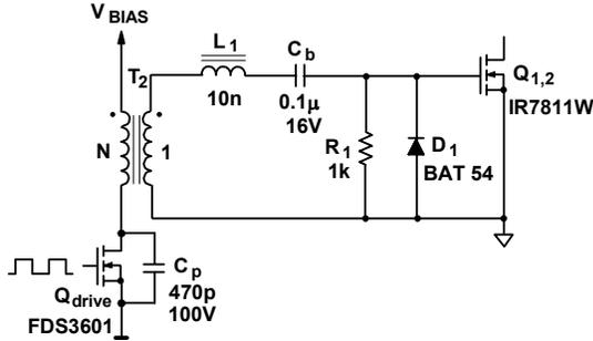
Fig. 12 Resonant gate drive circuit
