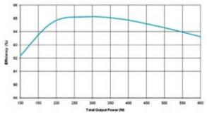
Figure 2: VRM Blade Efficiency (All six VRMs on Blade 1)
