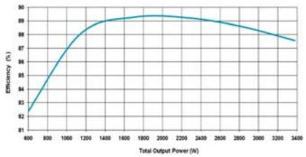
Figure 5: Total System Efficiency from 480VAC to 1VDC
