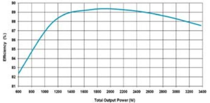
Figure 5: Total System Efficiency from 480VAC to 1VDC
