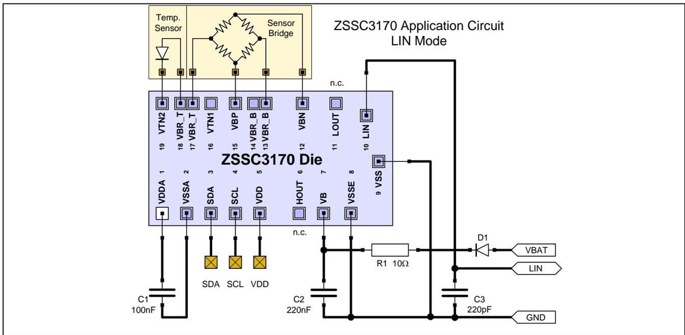
The ZSSC3170 can be directly connected to the battery in this application via the protective diode (D1) and current limiting resistor (R1) in applications where the maximum voltage drop does not exceed 1V. This circuit also requires a few external capacitors for noise immunity. In this schematic, the LOUT and HOUT pins are not connected and not used. The LIN interface requires a ground connection to the VSS pin.
