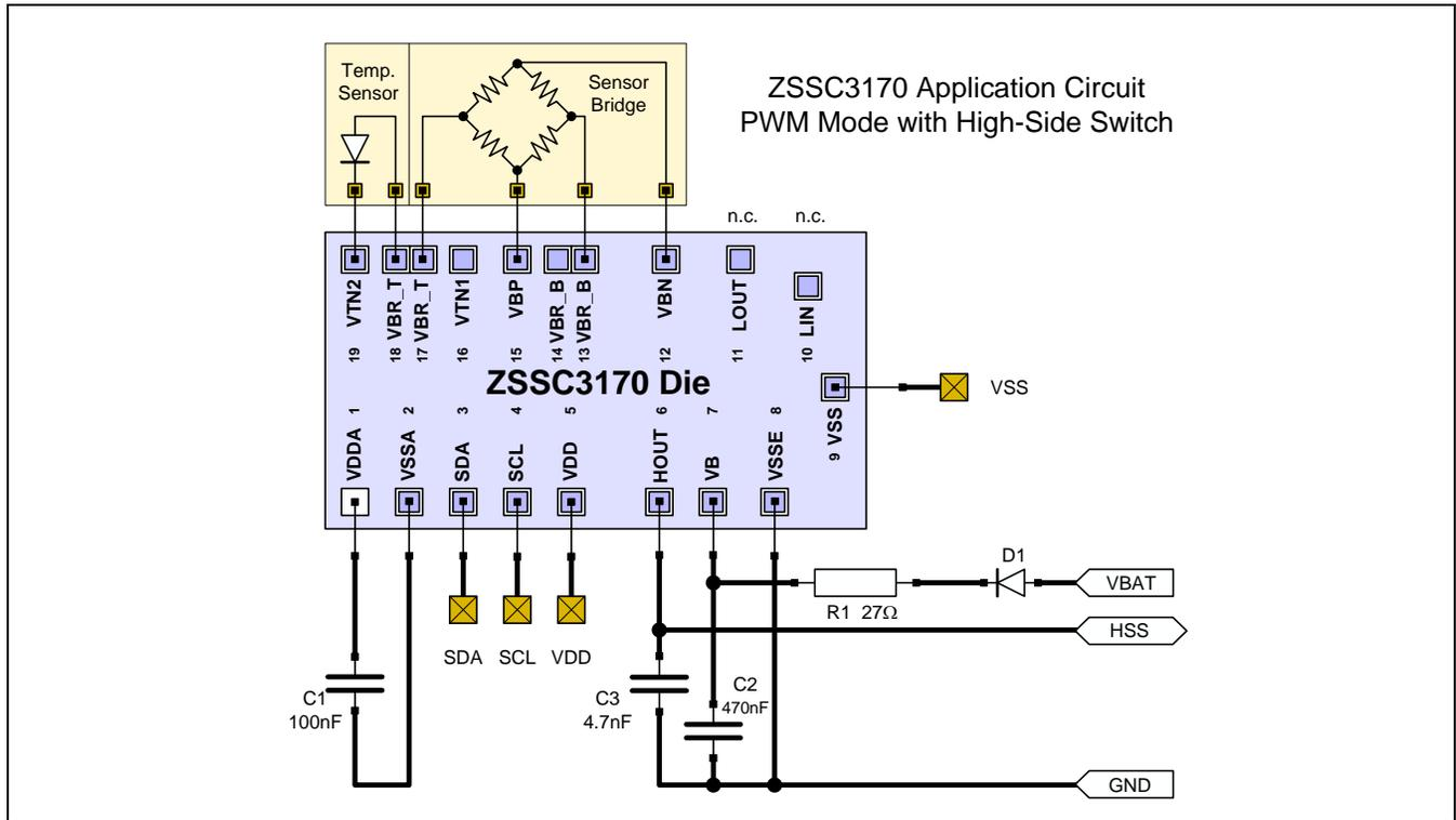
To setup and configure the ZSSC3170, the Command Mode must be entered during the startup window (30ms). Note that the HSS output on the HOUT pin has inverted signal levels due to the internal pull-down resistor.
