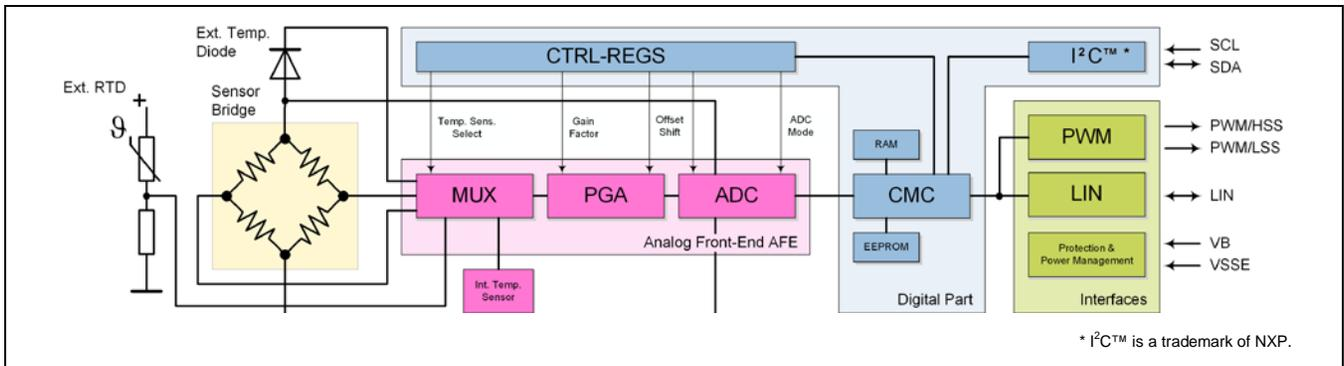
Figure 1.1 provides a block diagram of the ZSSC3170. An important advantage of this mixed-signal device is that noise sensitivity is greatly reduced because the calibration equipment and the ZSSC3170 are connected digitally.
