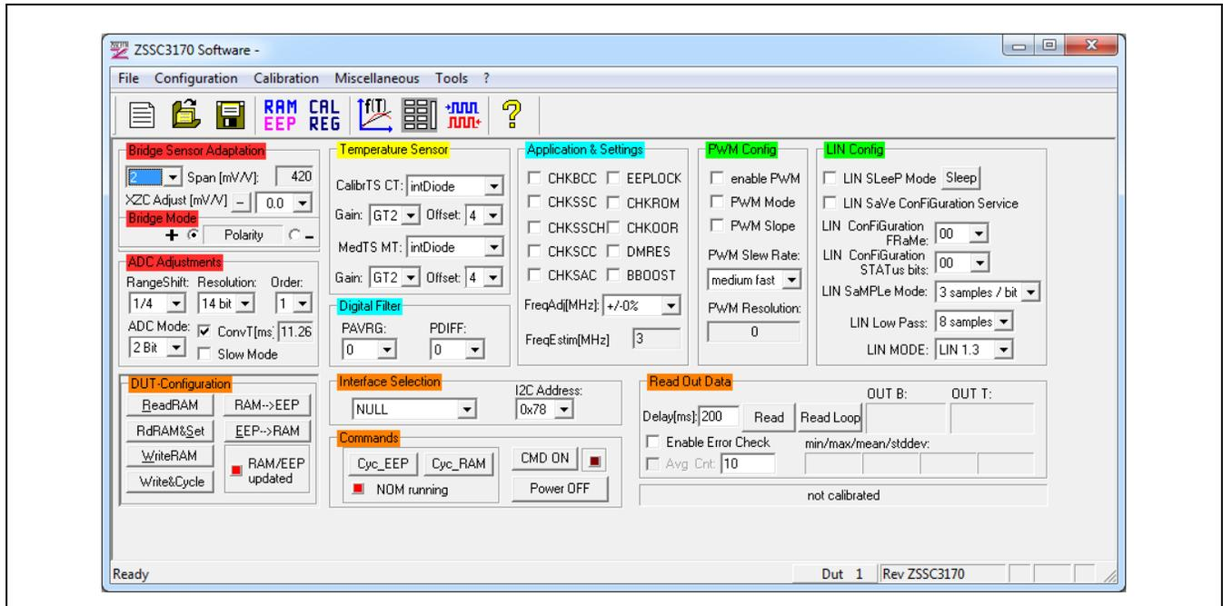
After the PWM is enabled, the signal limits should be defined in percentage of the maximum and minimum output value in the "Calibration" window of the software as shown in Figure 4.2.
