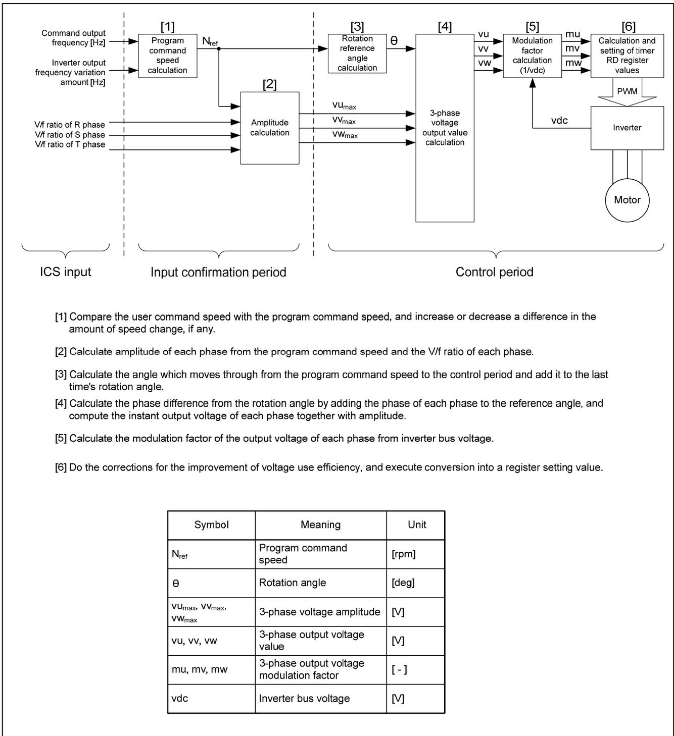
Figure 3-1 Control Flow of V/f Control
