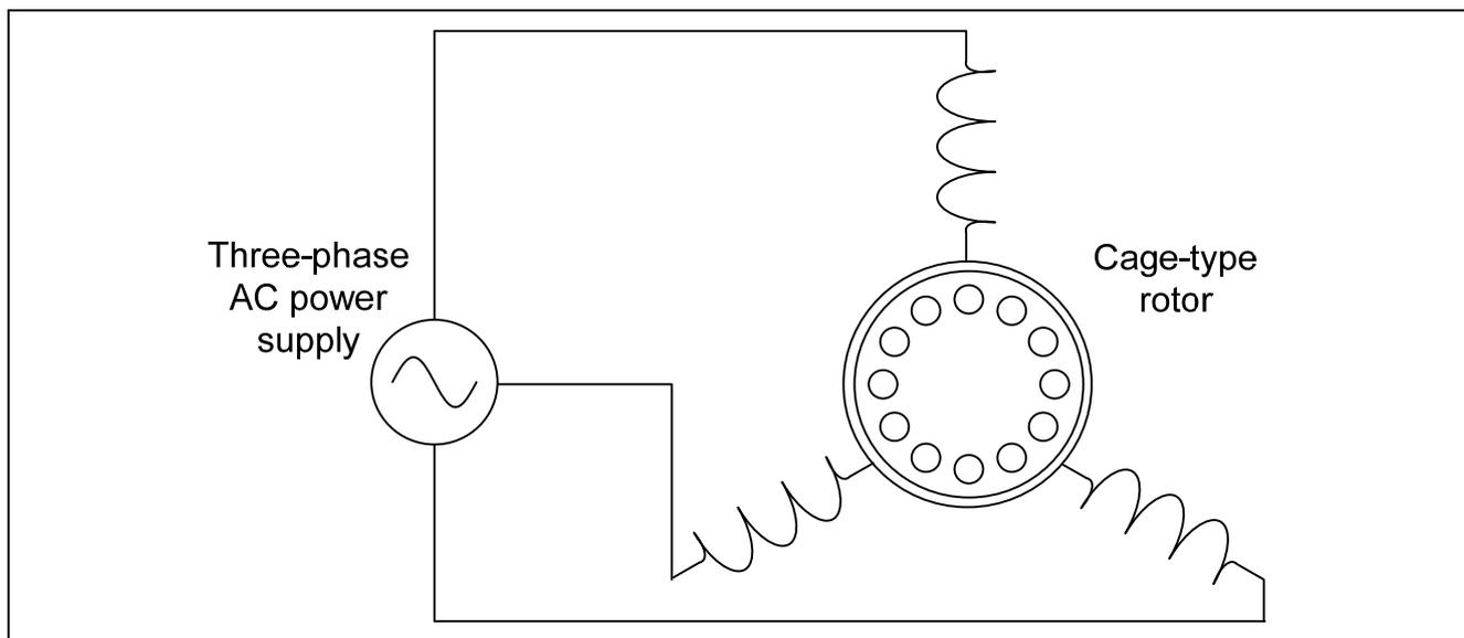
**Figure 2-1 Configuration Diagram of A Three-phase Induction Motor**
