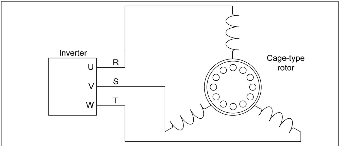
Figure 2-2 Configuration Diagram of Inverter Drive
