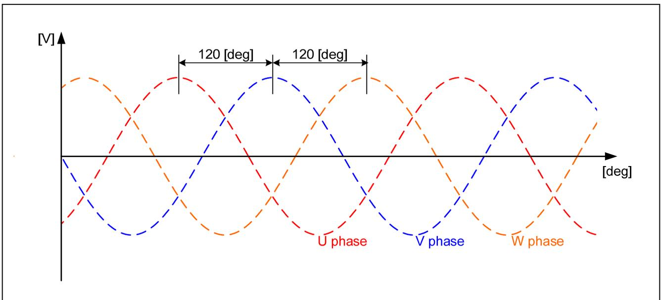
Figure 2-3 Three-phase Voltage Waveforms with 120-degree Phase Differences
