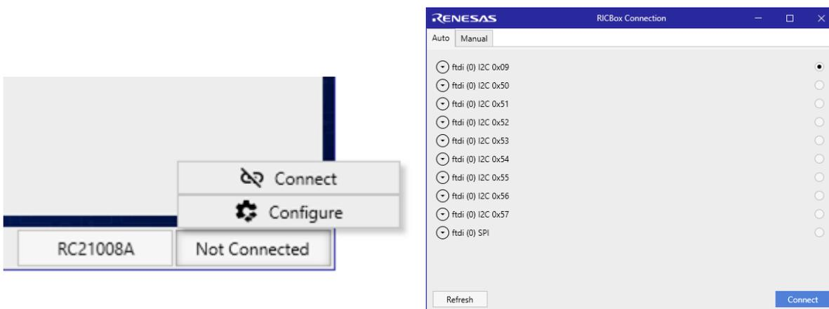
If the EEPROM is detected, then you are ready to program. Refer to the EEPROM user’s manual about which jumpers to set to add the EEPROM to the I<sup>2</sup>C bus.
