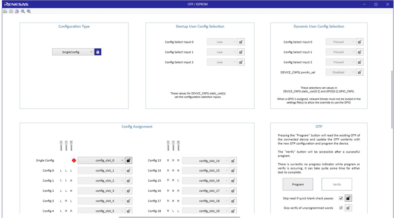
Notice the red error marker for “Single Config”. Click on the pull-down box and select the “default” config.
