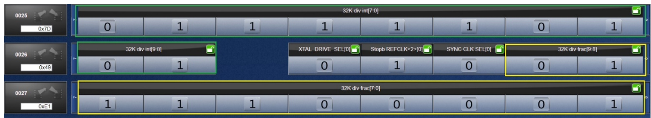
Figure 3. 25MHz Reference Input Divider Mode Register Setting from Timing Commander
