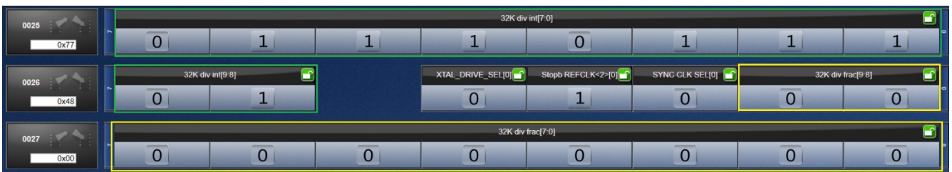
Figure 5. 24.576MHz Reference Input Divider Mode Register Setting from Timing Commander
