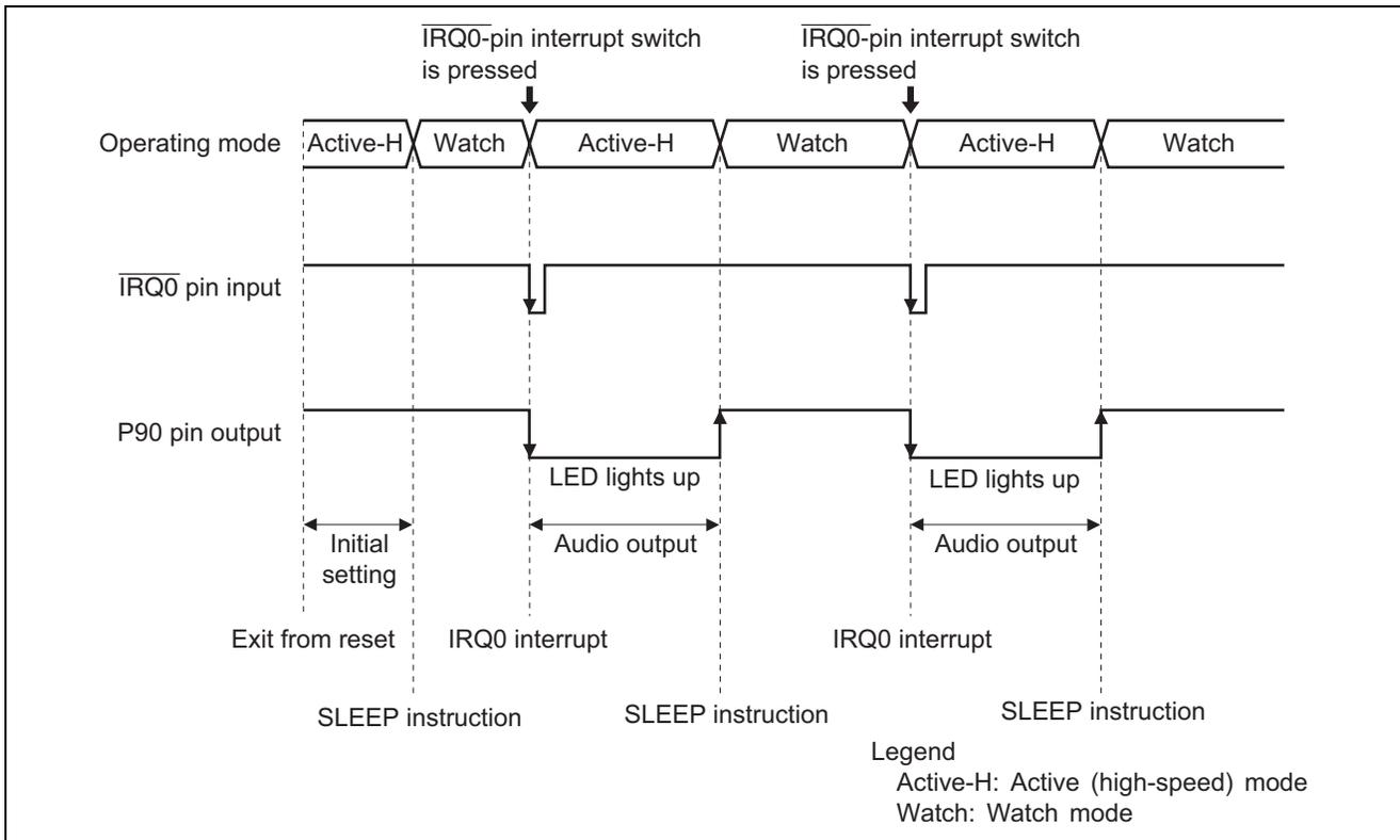
Figure 6 Audio-Output Operation
