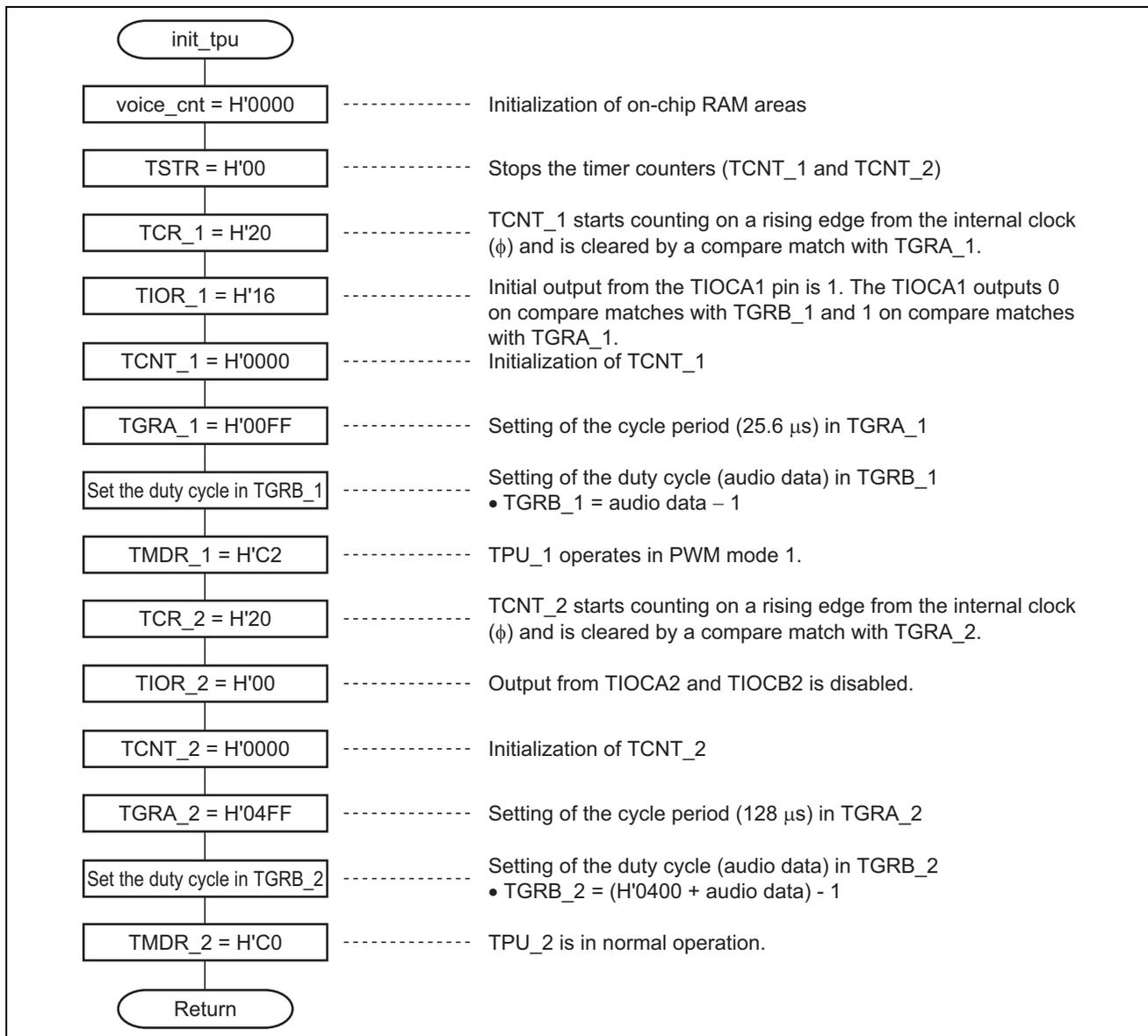
Figure 13 Flowchart of init\_tpu Function
