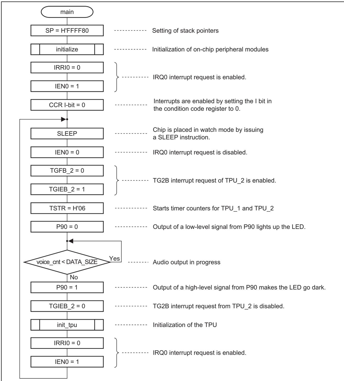
**Figure 9 Flowchart of main Function**
