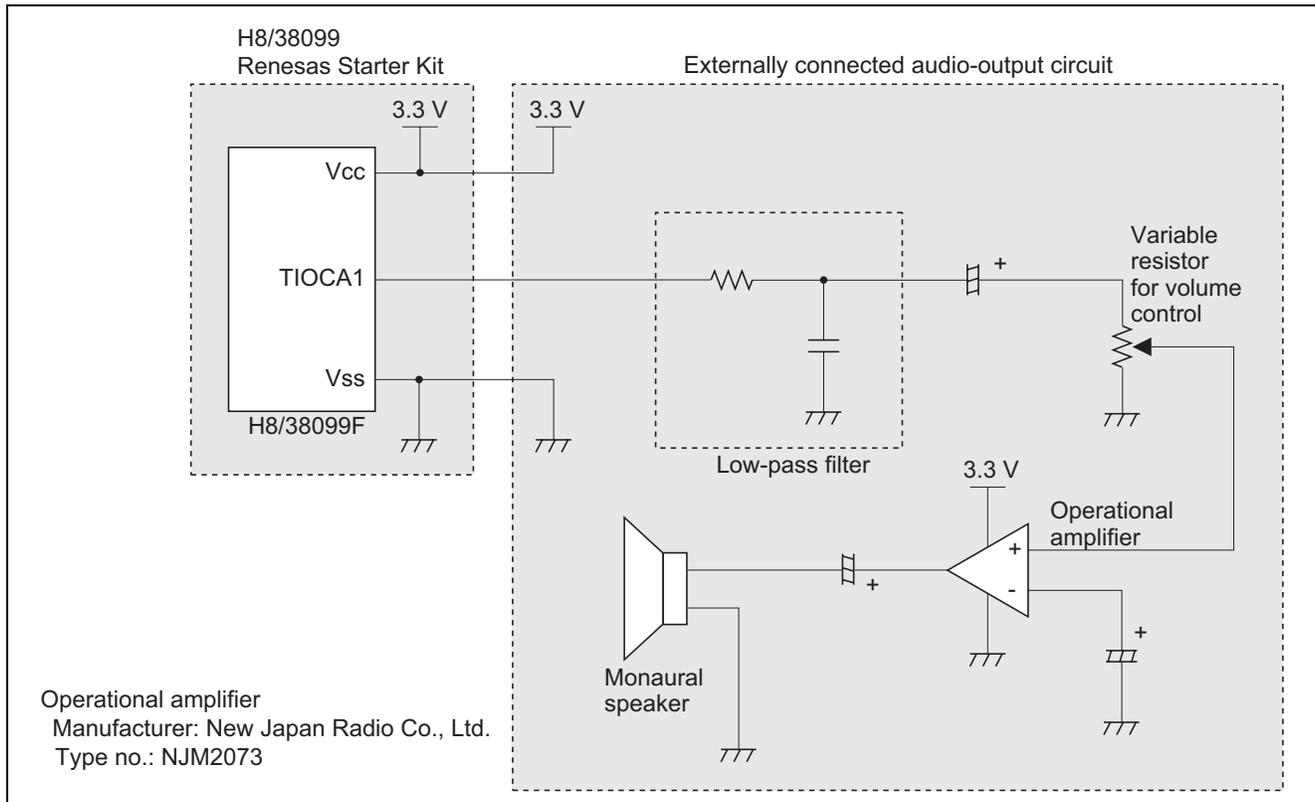
**Figure 3 Circuit Diagram of Audio Output**
