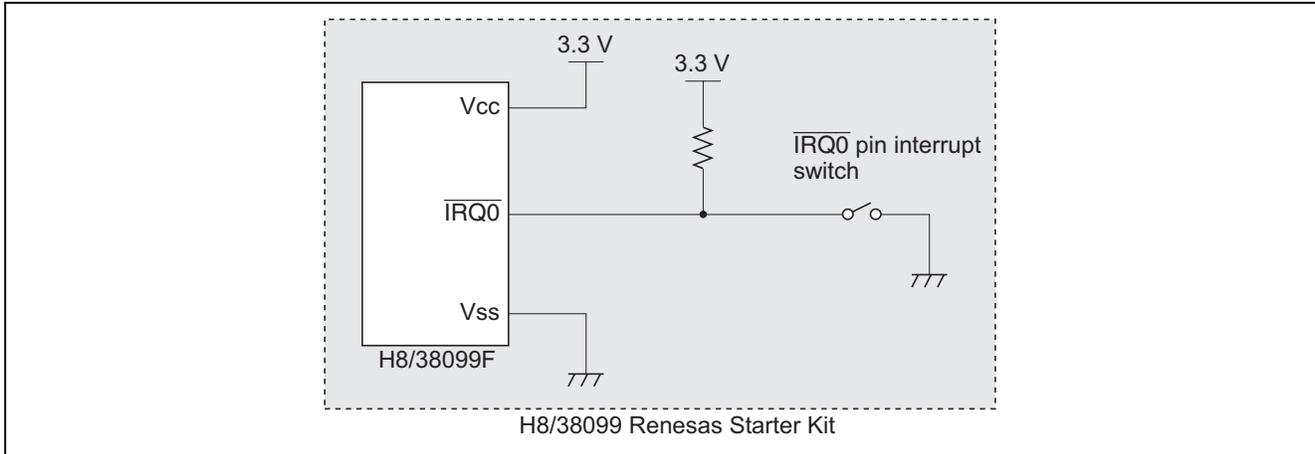
Figure 4 Circuit Diagram for the  $\overline{\text{IRQ0}}$  Pin Interrupt Switch
