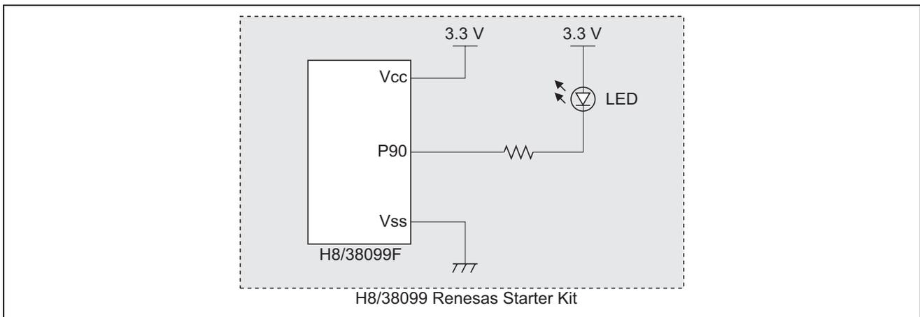
Figure 5 Circuit Diagram for the LED
