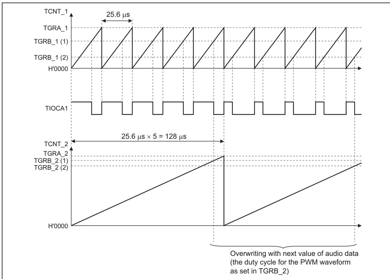
Figure 7 Operation of PWM Output by the TPU
