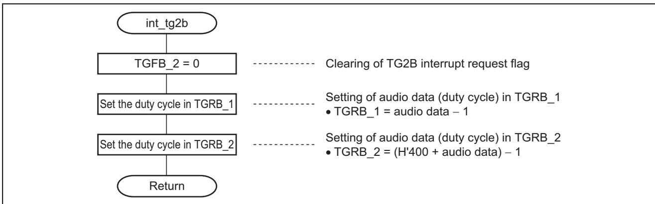
**Figure 11 Flowchart of int\_tg2b Function**
