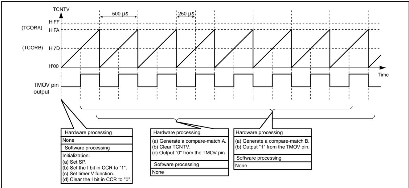
Figure 3.1 Operational Principle for TMOV Pin Output
