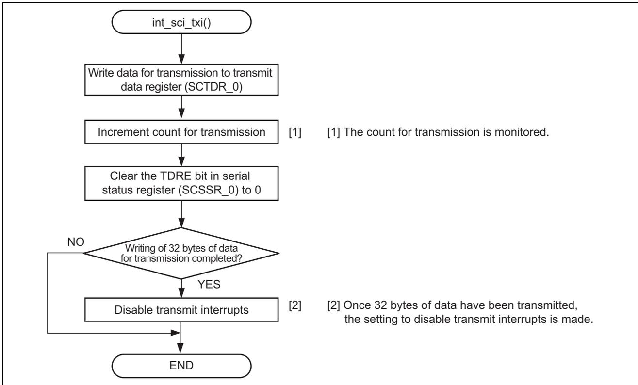
Figure 8 Flow for Handling Transmit Interrupts in Asynchronous Mode
