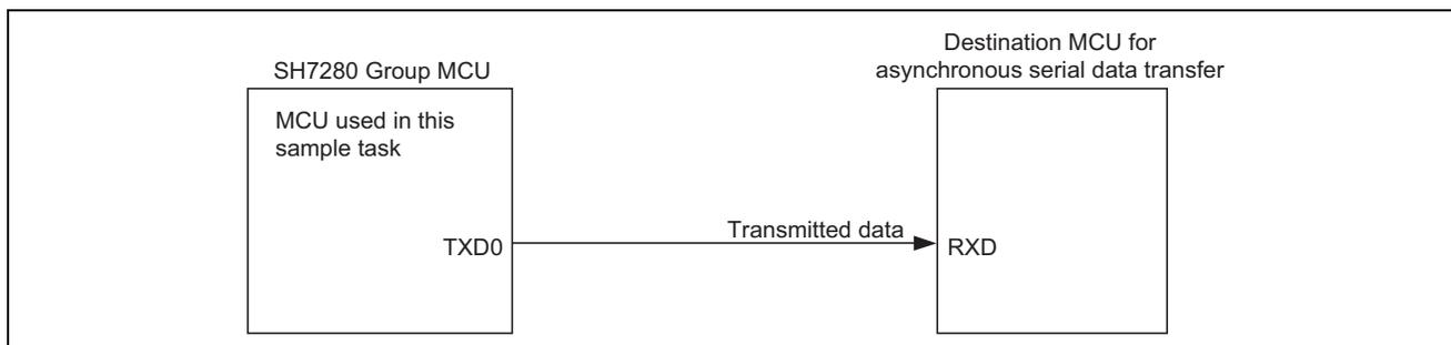
**Figure 1 Connection Example for Transmission by the SCI in Asynchronous Mode**
