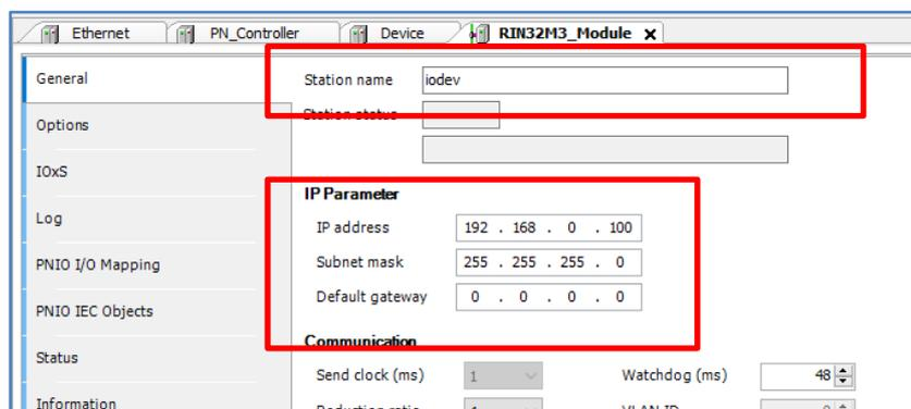
Figure 3.12 Stet Station Name and IP Address
