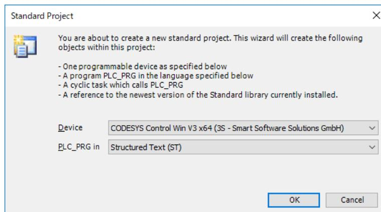
Figure 2.2 Select the Device and PLC programming
