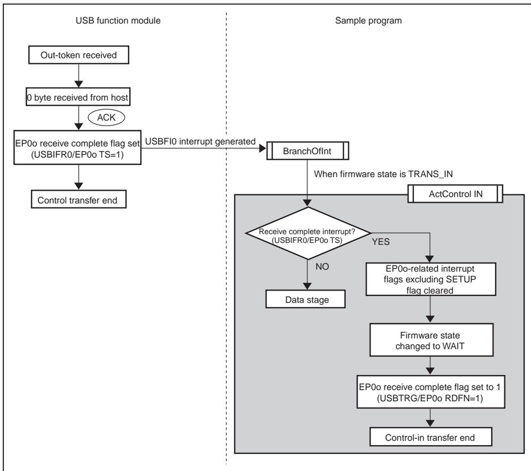
Figure 5.9 Status Stage (Control-In Transfer)
