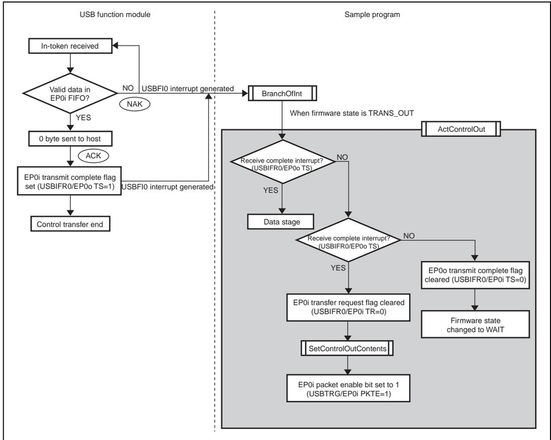
**Figure 5.10 Status Stage (Control-Out Transfer)**
