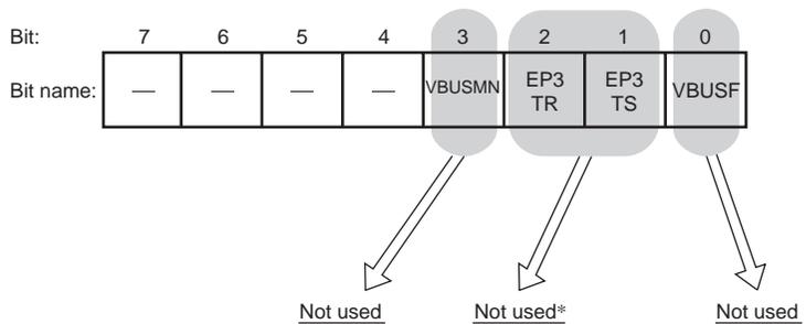
Note: Because this sample program does not support interrupt transfers, the interrupt associated with EP3 is not used.
