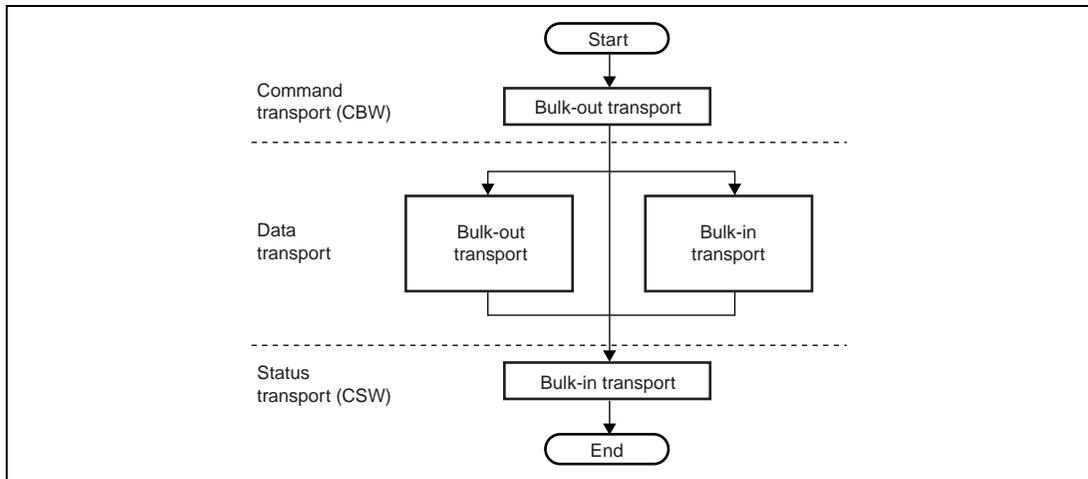
**Figure 2.1 Relationship between Transfer Methods and Transports**
