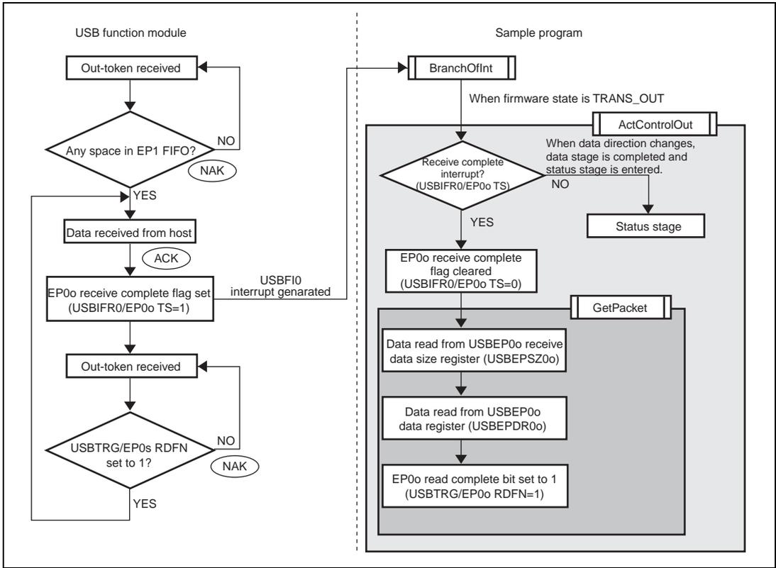
**Figure 5.8 Data Stage (Control-Out Transfer)**
