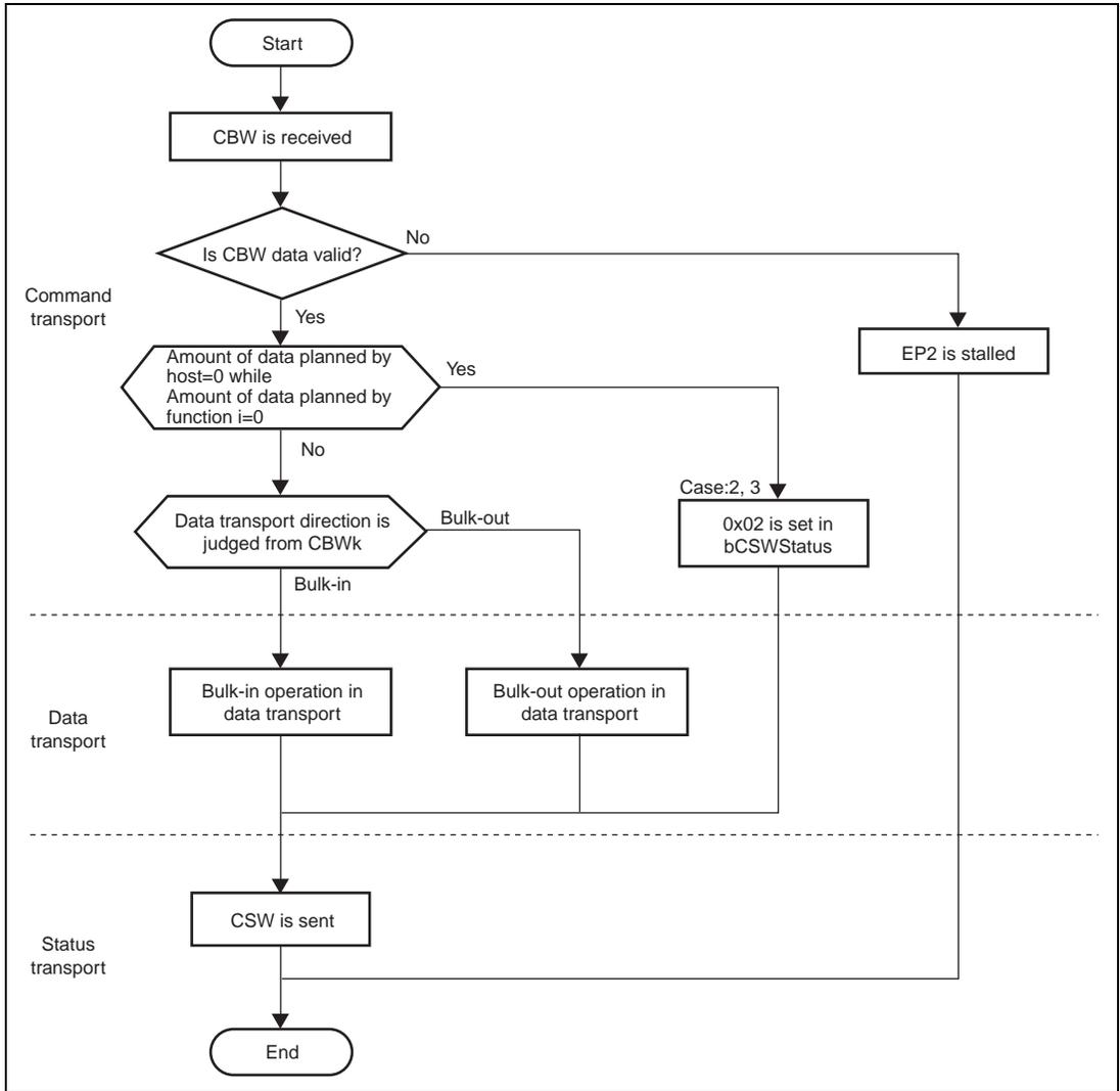
**Figure 4.6 Error Processing Flow in Data Transport (1)**
