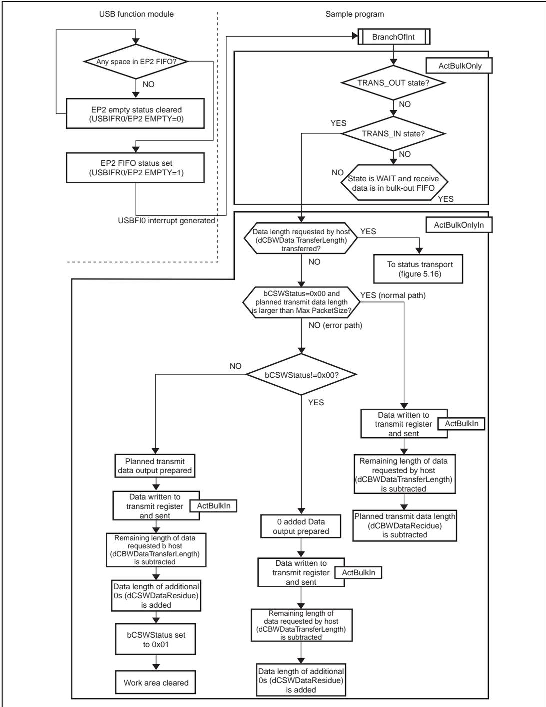
**Figure 5.14 Data Transport (Bulk-In Transport)**
