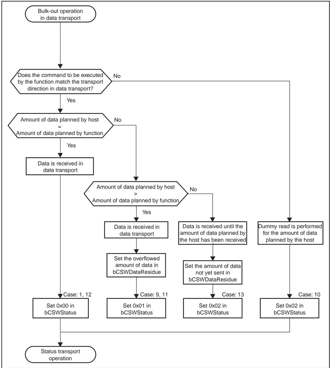
**Figure 4.8 Error Processing Flow in Data Transport (3)**
