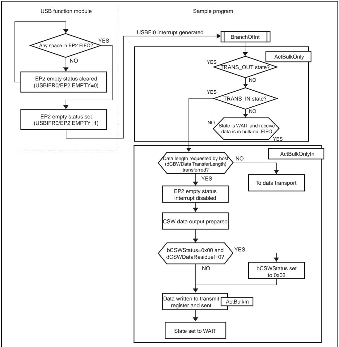
Figure 5.16 Status Transport (Data Transport Bulk-In Transport)
