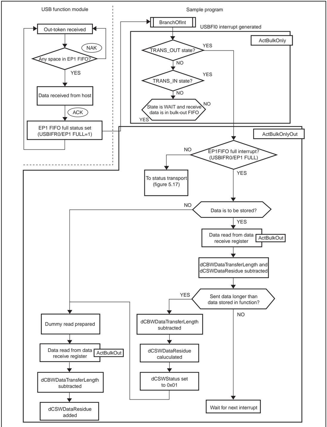
**Figure 5.15 Data Transport (Bulk-Out Transport)**
