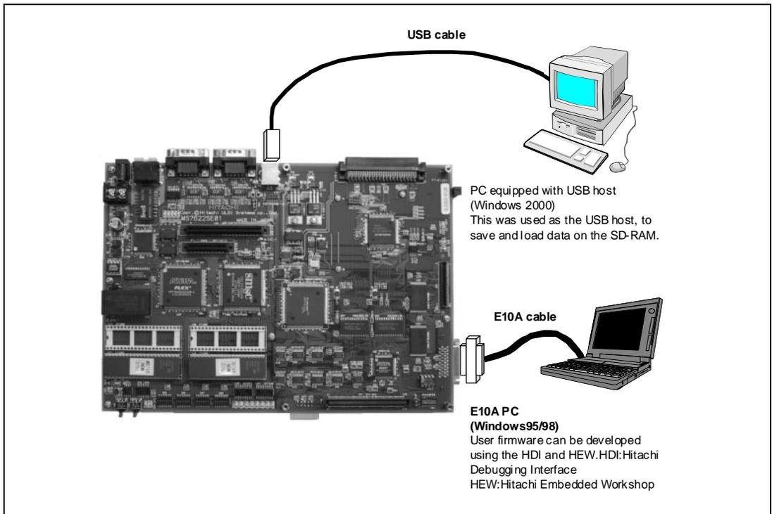
**Figure 3.1 Device Connections**
