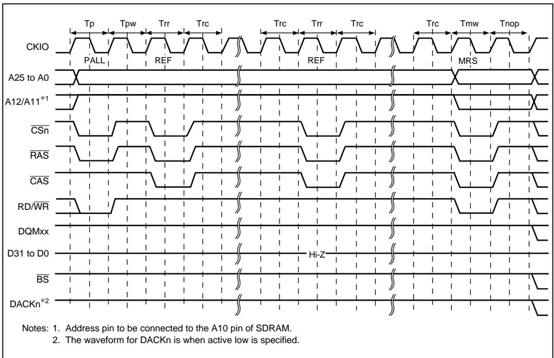
Figure 3.9 Synchronous DRAM Mode Write Timing (Based on JEDEC)
