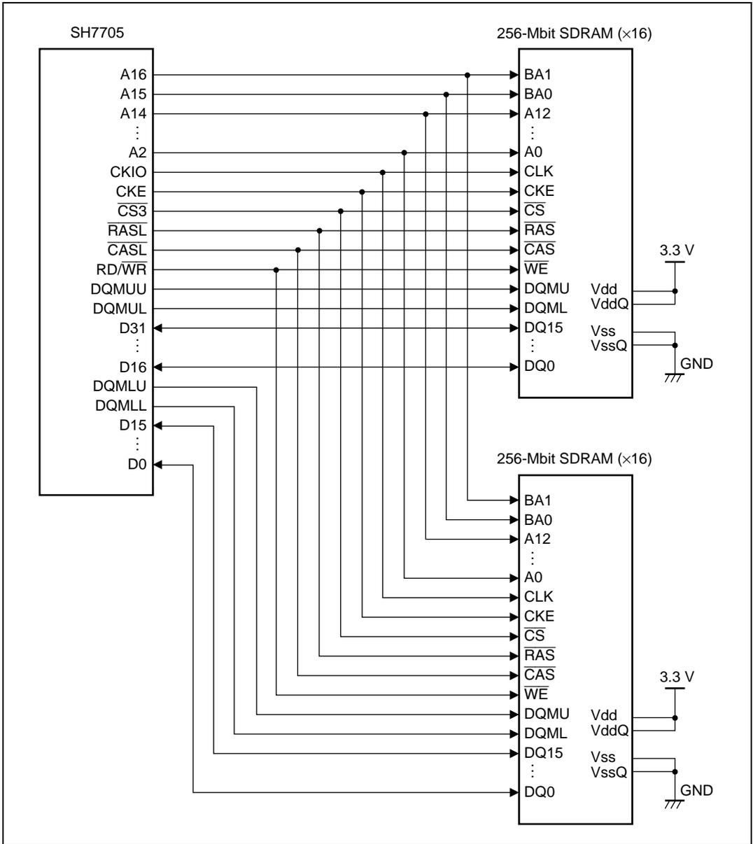
Figure 3.7 Block Diagram
