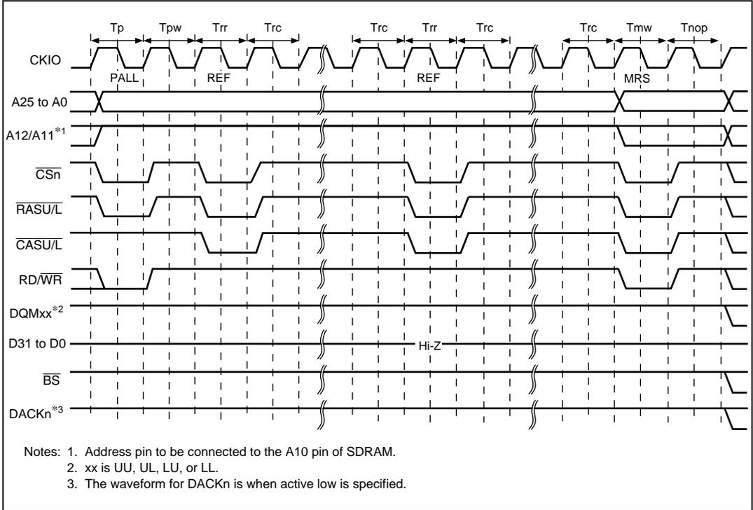
Figure 3.1 Synchronous DRAM Mode Write Timing (Based on JEDEC)
