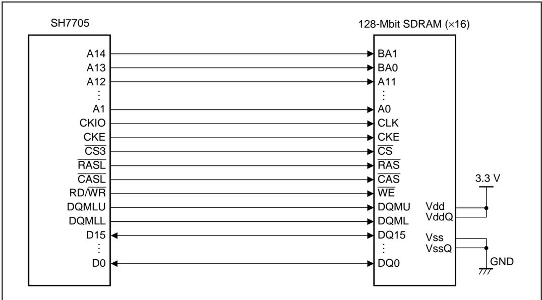
Figure 3.4 Block Diagram
