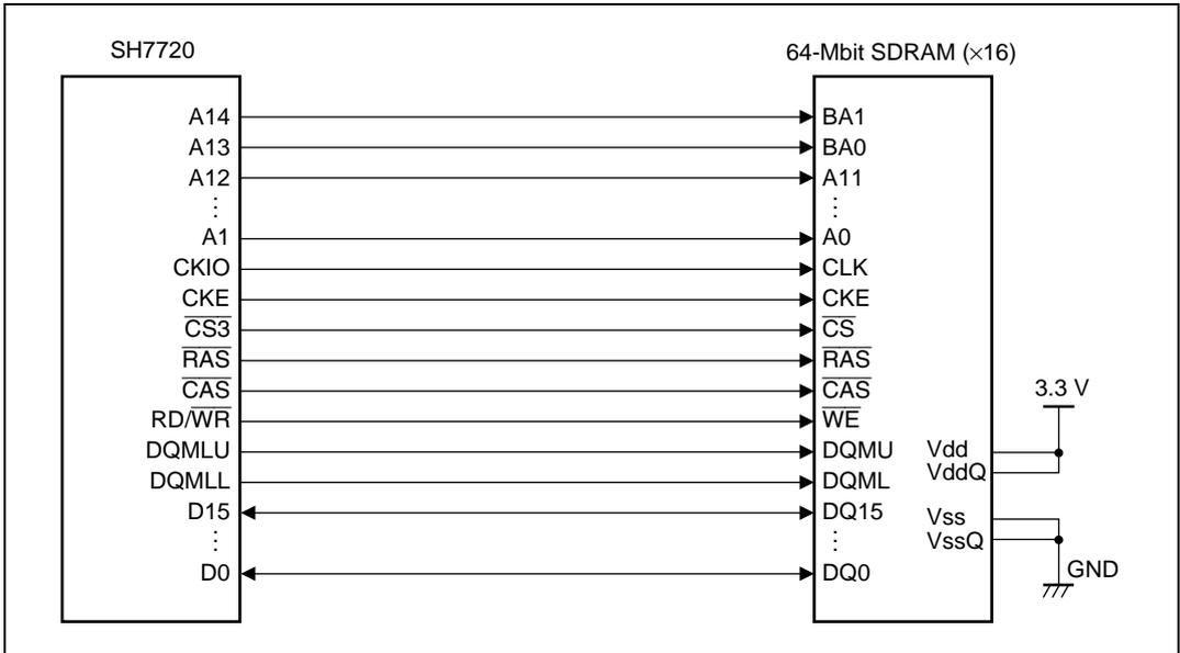
Figure 3.10 Block Diagram
