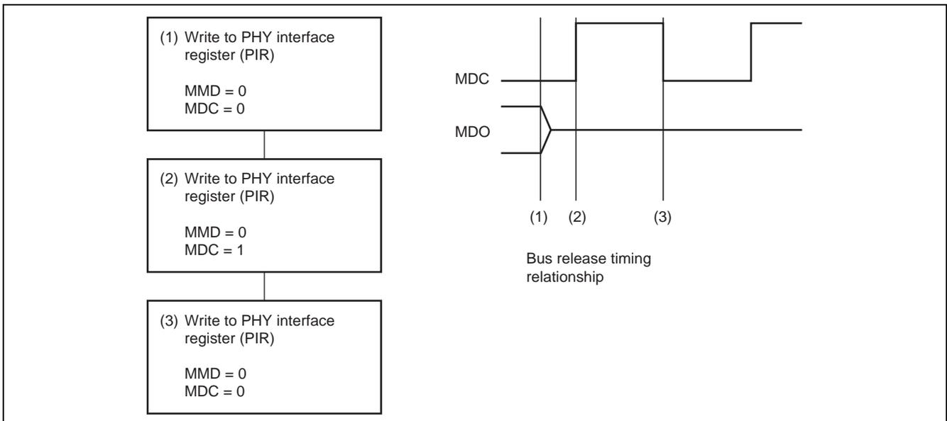
Figure 4 Flow of Bus Release (Z-output)
