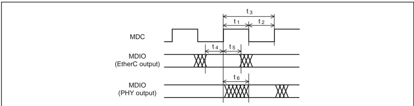
**Figure 6 MDC/MDIO Input/Output Timing**
