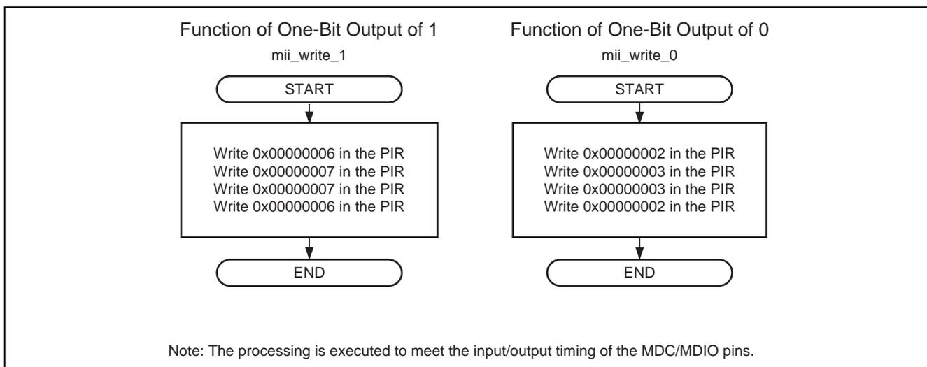
Figure 12 Flow of Processing to Access the MII Registers (4)
