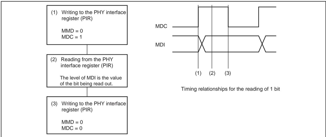
**Figure 5 Flow for Reading of One Bit**
