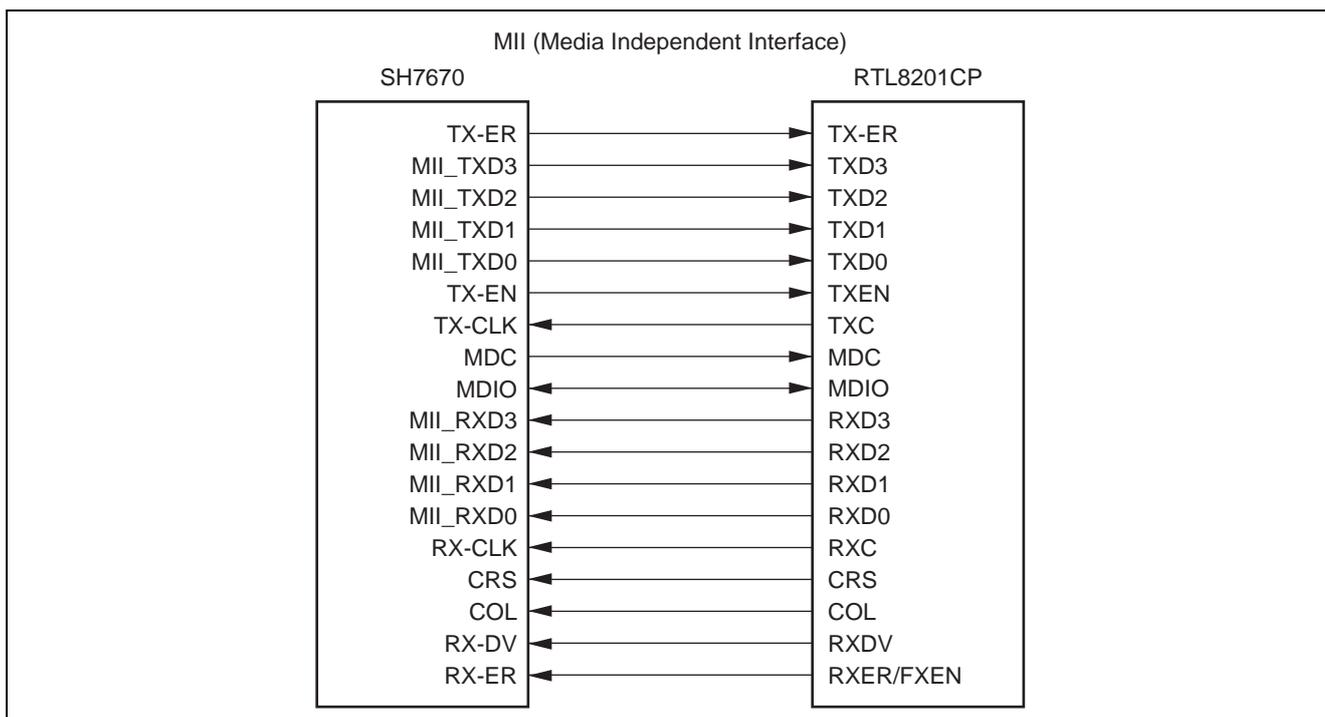
**Figure 1 Example of Connecting an MCU to the RTL8201CP**
